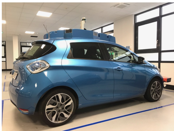
Figure 5.2: The ZoeCab data acquisition platform used to collect LIDAR objects ; the LIDAR sensor stands on top of the vehicle
