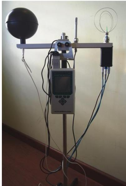
Figure 3-2. Thermal comfort measurement equipment.
