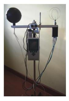
Figure 3-2. Thermal comfort measurement equipment.
