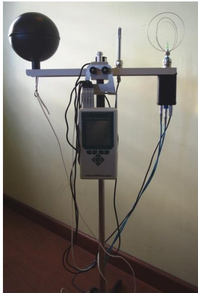
Figure 3-2. Thermal comfort measurement equipment.
