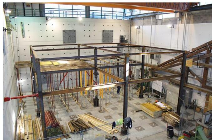
**Figure II.27:** Experimental test on 3D building frame structure (Zandonini et al., 2014).
