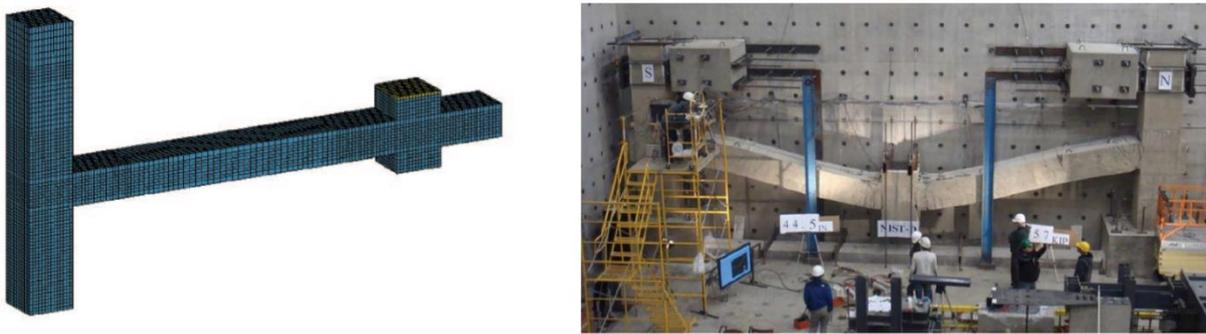
**Figure II.16:** Computational and experimental assessment of RC beam-column assembly under a column removal scenario (Sadek et al., 2011).
