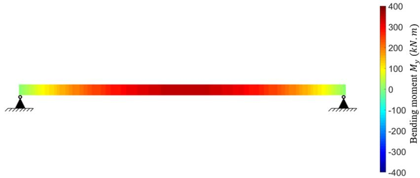
**Figure III.21:** Bending moment according to the static approach of yield design calculation (configuration B1).
