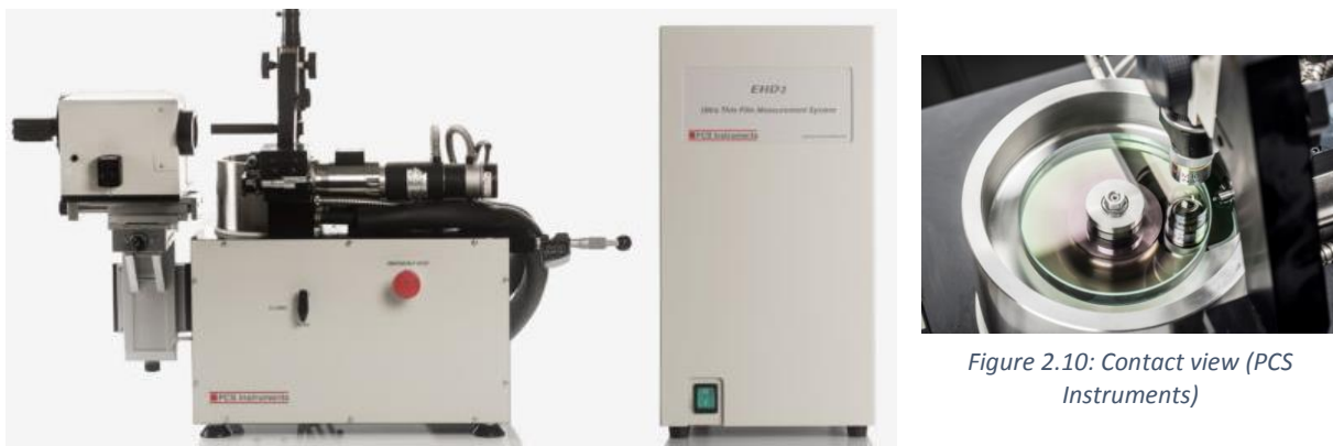
Figure 2.9: EHD2 from PCS Instruments (PCS Instruments)
