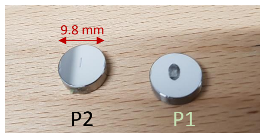
Figure 5.6: comparison between sample after HFRR test condition 5
