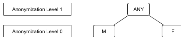
Figure 3.3: Anonymization hierarchy for the domain 'sex'. The scope of original values at the anonymization level '0' is limited. The anonymization of the original value leads to the replacement of it with 'ANY' denoting a generic upper class for both 'M' for male and 'F' for female.
