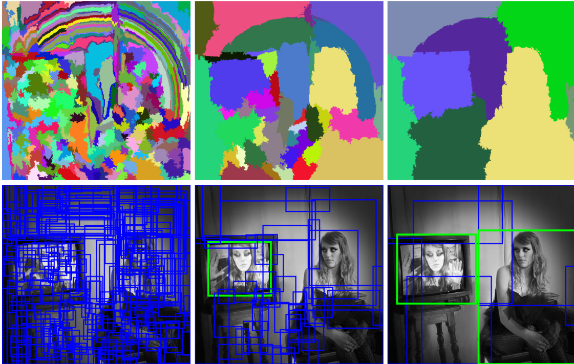
Figure 2.5 An example of selective search process, copied directly from [103]. Regions are proposed via bottom-up perceptual grouping.
