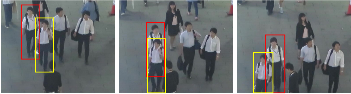
Figure 4.4 Example of adjacent similar looking people in MOT16 benchmark [67]. They are difficult for appearance models to distinguish. Once their trajectories cross, motion models are more robust for preventing mismatches or trajectory merging.
