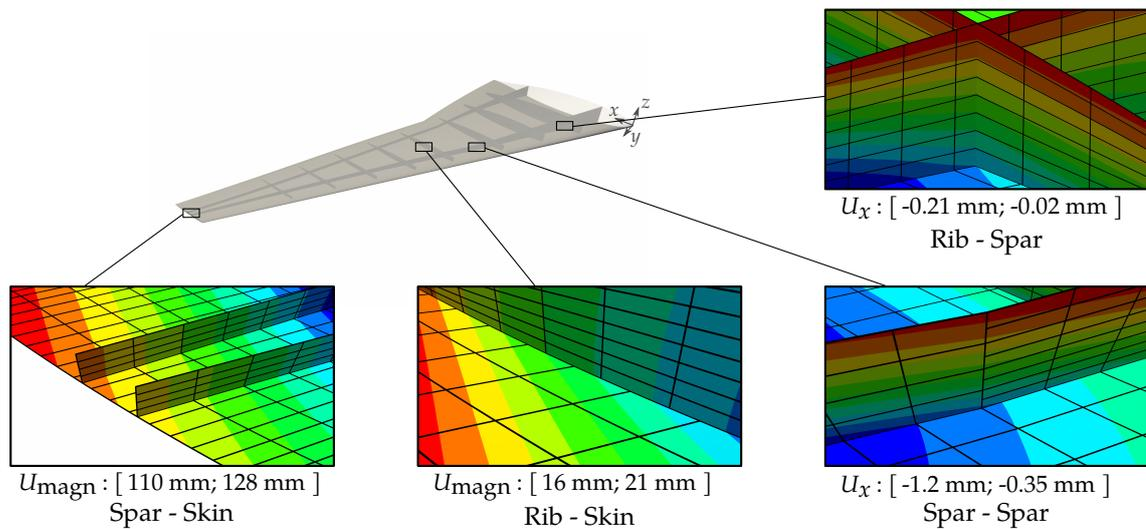
Figure 6.7 – Structural analysis of the CRM wing.
