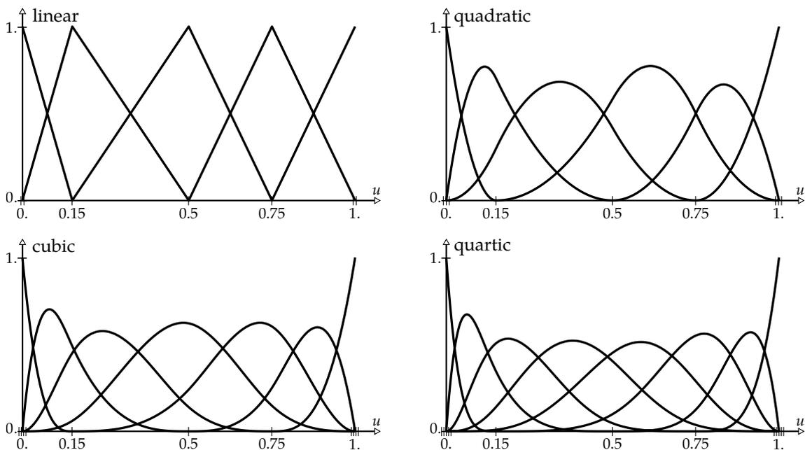
Figure 2.13 – Examples of B-Spline basis functions of different degree. Same interior knots were used (0.15, 0.50, and 0.75).
