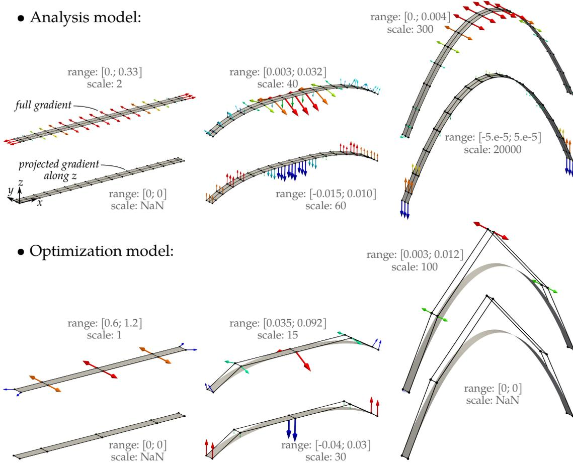
**Figure 3.18** – Sensitivity analysis for the arch. The planar beam (left) leads to a zero gradient and thus cannot be taken as the initial configuration. In the optimal configuration (right), the  $z$ -component of the gradient is also null which reflects that a minimum has been found.
