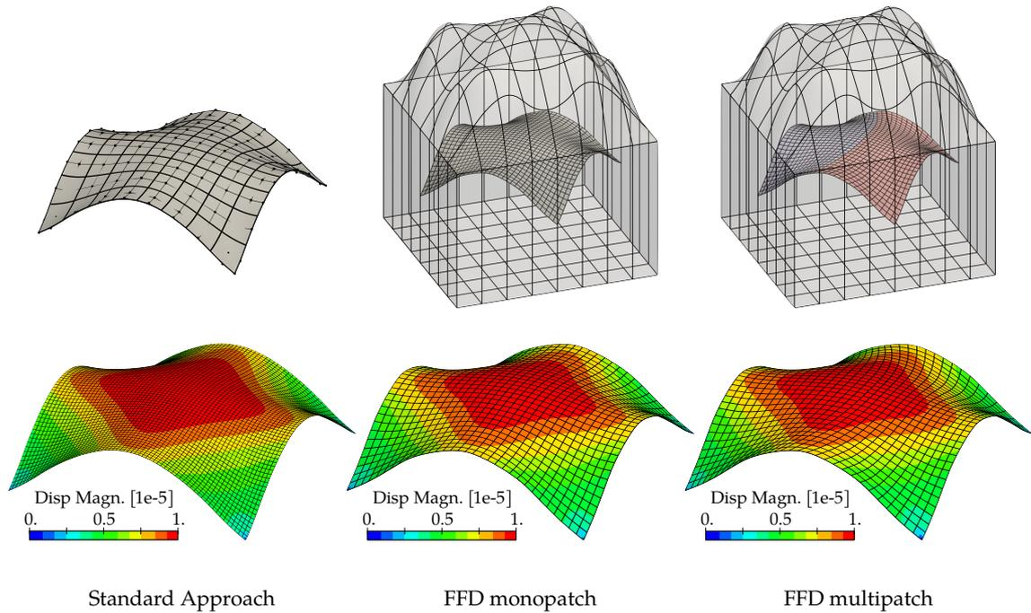
**Figure 5.20** – Comparison of the results obtained for the shape optimization of the square roof. The FFD approach applied to the multipatch model gives very similar results than both monopatch resolutions (standard and FFD).
