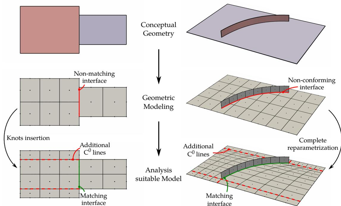
**Figure 4.1** – NURBS modeling generates multipatch geometries where each patch represents a specific part of the complete structure. Naturally, these patches present non-matching or even non-conforming parametrization at their interfaces. Additional procedures are required to get a final model with conforming and matching interfaces.
