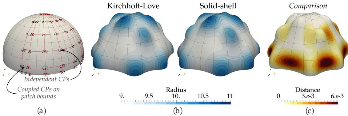
**Figure 3.22** – Shape optimization of the pinched hemisphere: (a) 25 design variables update the optimization model, (b) final shapes obtained by both shell formulations, and (c) comparison of the final shapes depicted as the distance between their mid-surface.
