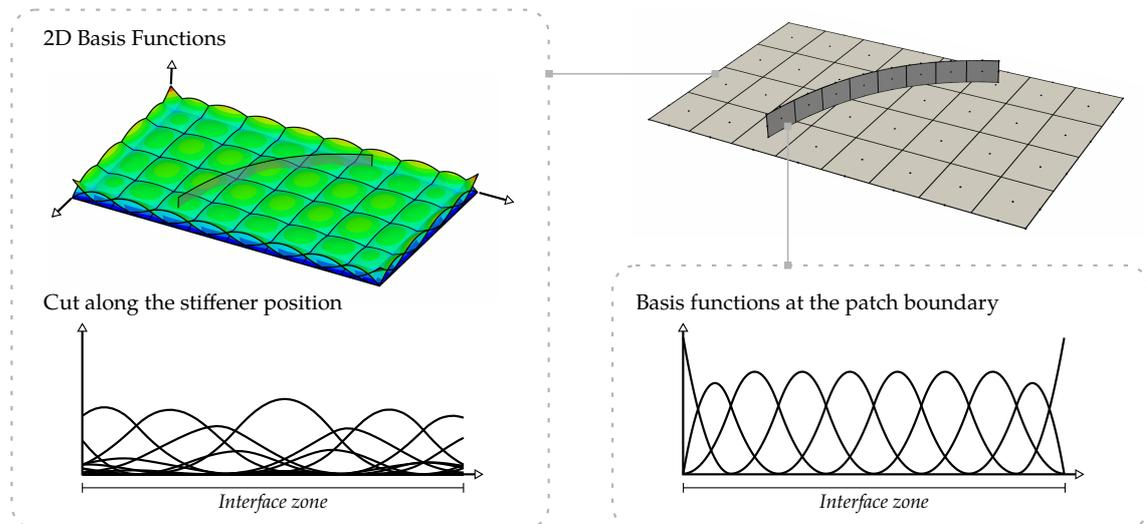
**Figure 4.3** – Example of a stiffened panel with non-conforming parametrizations: the interface crosses the elements from the panel. The trace spaces of both sides are particularly different.
