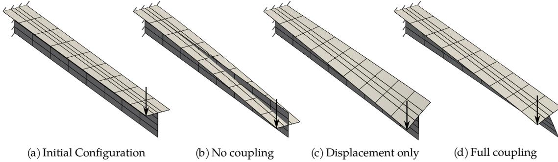
**Figure 4.5** – Kinematic constraints for Kirchhoff–Love shells: at the patch junction, the three components of the displacement fields need to be coupled (c). Additionally, the continuity of the rotation in the tangent direction of this interface curve is imposed (d).
