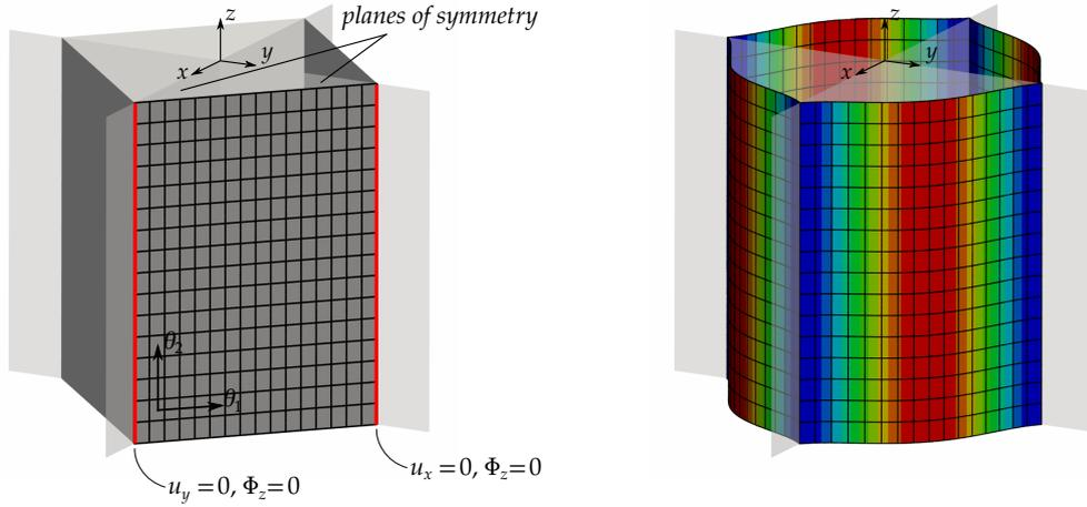
**Figure 4.9** – Single patch model of a square shape tube under internal pressure: the constraints for the rotation on the patch edges are imposed through the Mortar coupling operators. Looking at the deformed configuration shows that the angles between the patch and the planes of symmetry are kept fixed (right side, color map corresponds to the displacement magnitude).
