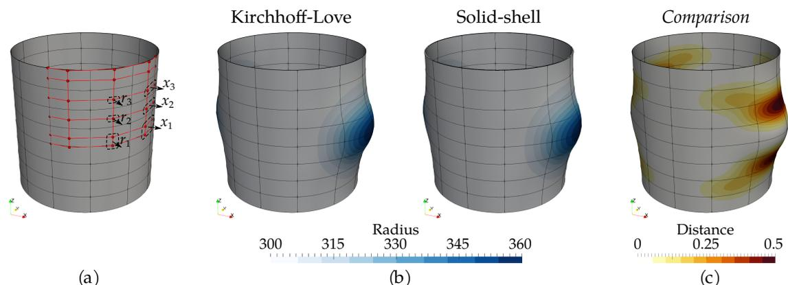
**Figure 3.21** – Shape optimization of the pinched cylinder: (a) 6 design variables update the optimization model, (b) final shapes obtained by both shell formulations, and (c) comparison of the final shapes depicted as the distance between their mid-surface.
