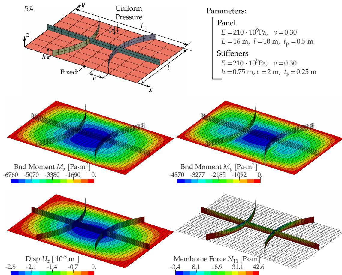
**Figure 4.20** – Description and results for the stiffened panel problem. It consists in the assembly of a rectangular plate with three stiffeners; two with a parabolic shape crossed by a straight one. It leads to four non-conforming patches and five coupling interfaces (three stiffener/panel and two stiffener/stiffener interfaces). The main stress resultants for the panel are the bending moments whereas the stiffeners are mainly subjected to membrane forces.
