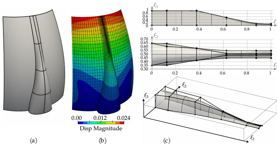
**Figure 6.13** – Optimal configuration of the stiffened curved wall: (a) final geometry and (b) the magnitude of the displacement. (c) The final embedded surface: side, top views and 3D views. The 2D views give information on the coordinates of the control points.
