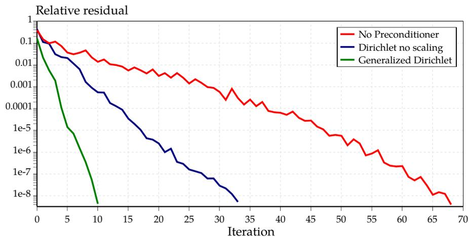
**Figure 4.17** – Convergence of the dual DD solver when applied to the heterogeneous beam problem with five sub-domains 2A (refinement level 4 according to table 4.3). The scaling step of the generalized Dirichlet preconditioner improves drastically the convergence rate.
