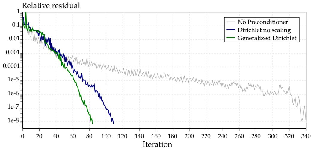
**Figure 4.21** – Convergence plot of the dual DD solver when applied to the stiffened panel 5A (refinement level 2 according to table 4.6). Without the preconditioning step, the solver faces difficulties to converge. The scaling of the generalized Dirichlet preconditioner accelerates the convergence in comparison with the classical Dirichlet preconditioner.
