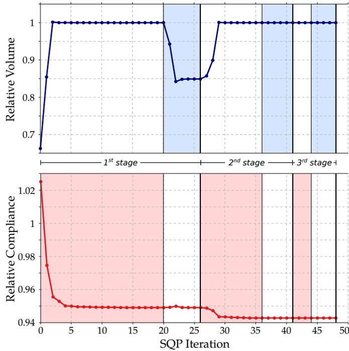
**Figure 3.26** – Optimization history of the bi-step approach applied to the stiffened cylinder problem. Three global iterations with successive shape and sizing steps are performed until convergence. Red zones denote the shape steps where the compliance is minimized and blue zones denote the sizing step where the volume is minimized.
