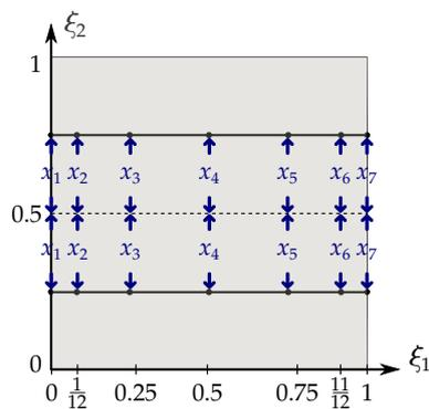
**Figure 5.15** – Settings of the shape optimization problem of the partly clamped hyperbolic paraboloid with stiffeners. Seven design variables  $x_i$  are associated to the embedded surfaces in order to impose shape changes to the stiffeners.
