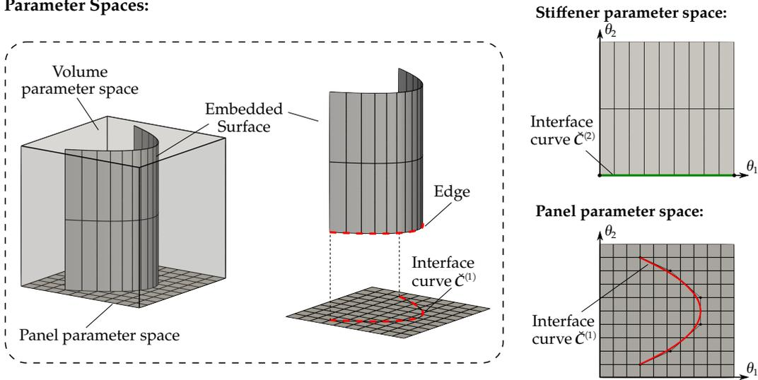
**Figure 5.13** – Definition of the interface curves with the embedded approach. For the stiffener, the interface curve  $\check{C}^{(2)}$  lies on one edge of the embedded surface. For the panel, the interface curve  $\check{C}^{(1)}$  can be extracted from the embedded surface.
