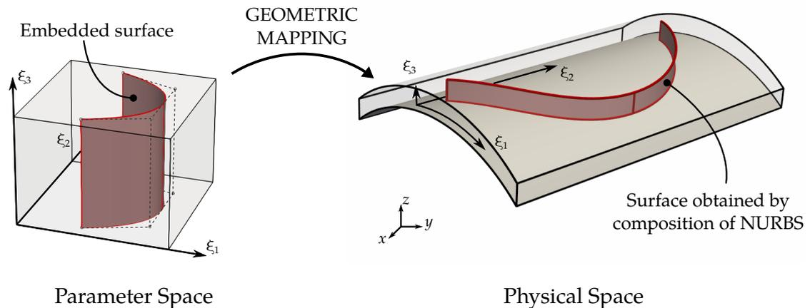
**Figure 5.3** – Construction of a stiffened structure using embedded surfaces. The final surface describing the stiffener is obtained by the composition of a NURBS surface and a NURBS volume. This construction ensures that the stiffener is perfectly lying on the portion of cylinder.
