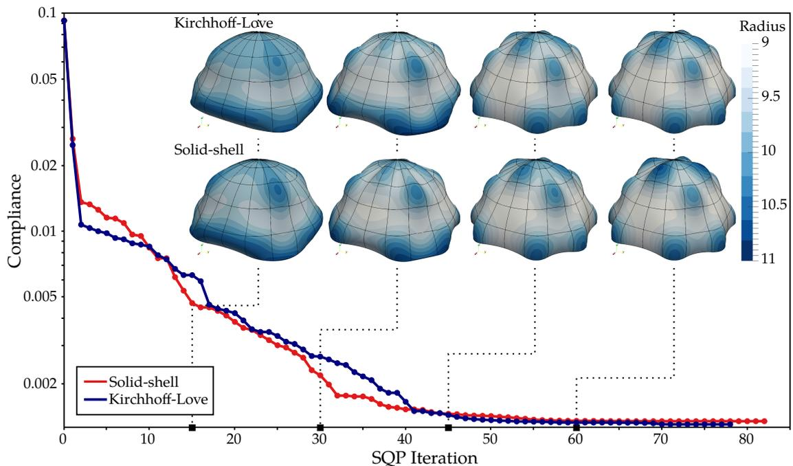
**Figure 3.23** – History of compliance and shape during the optimization of the pinched hemisphere when using Kirchhoff–Love NURBS shell elements and NURBS-based Solid-shell elements.
