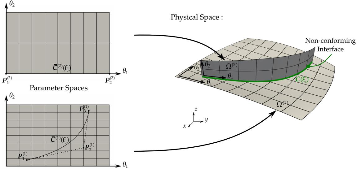
**Figure 4.6** – Non-conforming parametrization: the interface between both surfaces is represented in their parameter spaces by using NURBS curves  $\bar{C}^{(s)}$ . These curves are generated in order to ease the building of the coupling operators for the Mortar approach.
