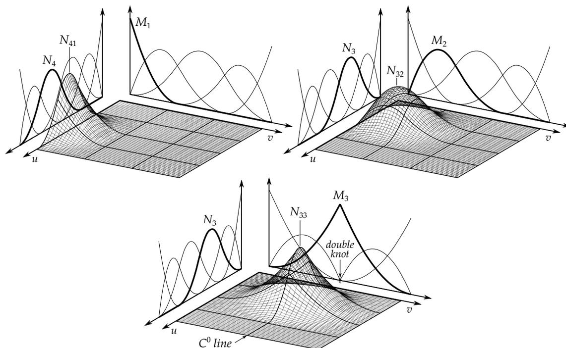
**Figure 2.16** – Example of bivariate B-Spline basis functions. The lower continuity at repeated knots of the univariate basis functions propagates along the knot lines due to the tensor product.
