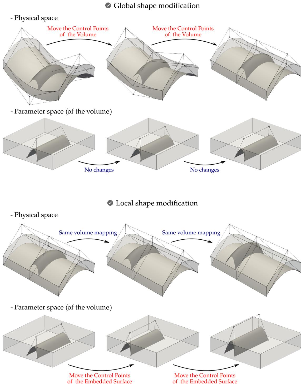
**Figure 5.5** – Using NURBS compositions offers two possibilities for imposing shape deformations. By modifying the volume, one can act on the global shape. By acting on the embedded entities, one can modify specific parts, as for instance the stiffeners. The bonding condition at the interfaces are automatically satisfied.
