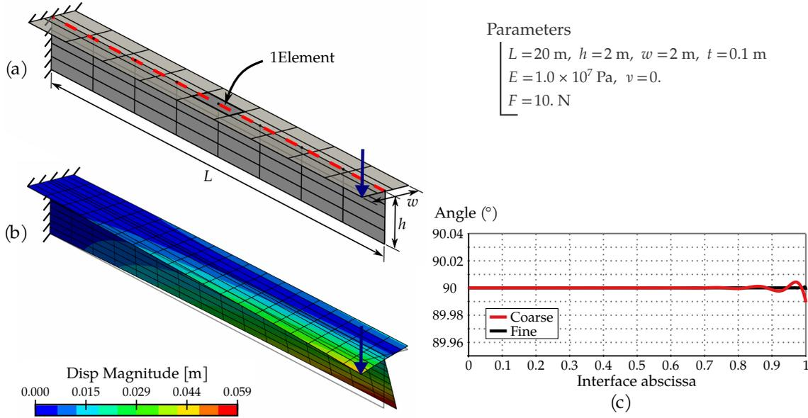
**Figure 4.8** – T-Beam non-matching coupling: (a) Description of the problem: the interface cuts the upper patch at the middle of some elements. (b) Deformed configuration with scale factor of 10 and the magnitude of the displacement field. (c) Angle between the patches along the interface after deformation. Coarse case corresponds to the mesh depicted in (b). Fine mesh is three times refined.
