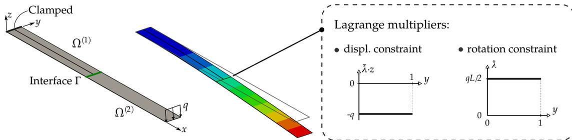
**Figure 4.7** – Cantilever beam with end load: the beam is decomposed in two non-matching patches and coupled with the Mortar approach. The shape of Lagrange multipliers for the displacement and the rotation continuity constraints are shown on the right.
