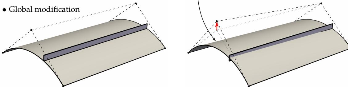
**Figure 5.2** – Moving a stiffener lying on a portion of cylinder. Imposing the shape update in non-planar directions is challenging due to the violation of the bonding condition.
