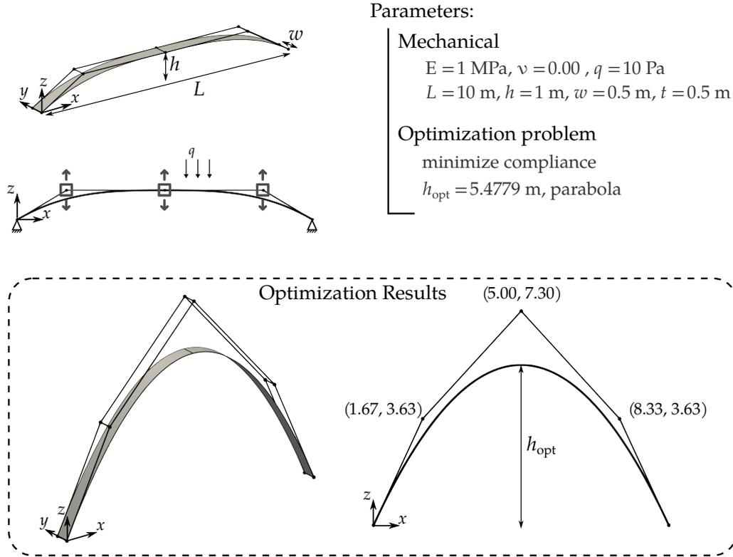
**Figure 3.17** – Settings for the shape optimization of an arch under constant load. The optimal result is a parabola with a specific height to length ratio [72].
