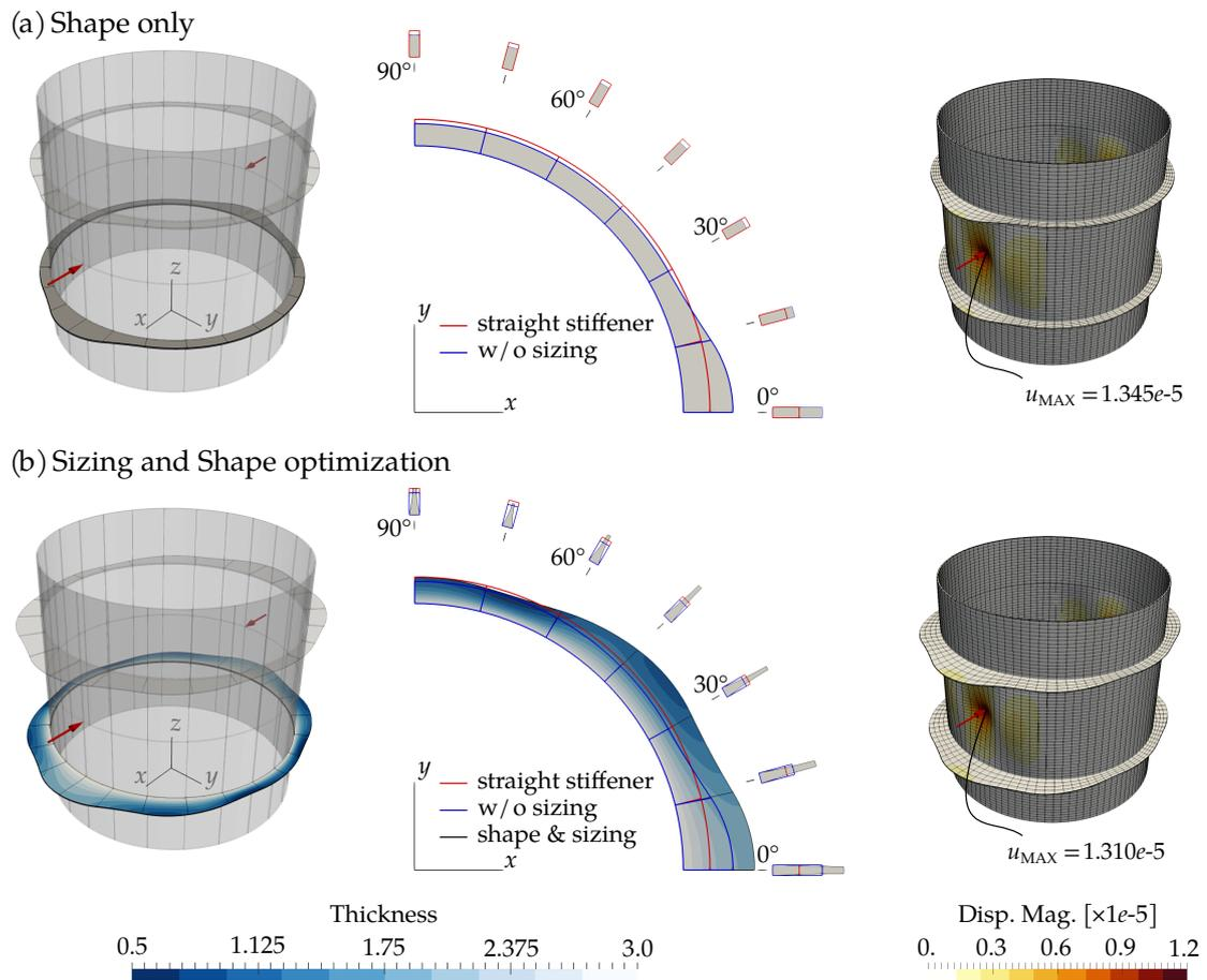
**Figure 3.25** – Optimization results of the stiffened cylinder: (a) final shape when only the stiffener height is modified, and (b) final shape when both height and thickness are optimized (annotations on figure 3.24 can be helpful to understand the detailed views of the stiffener).
