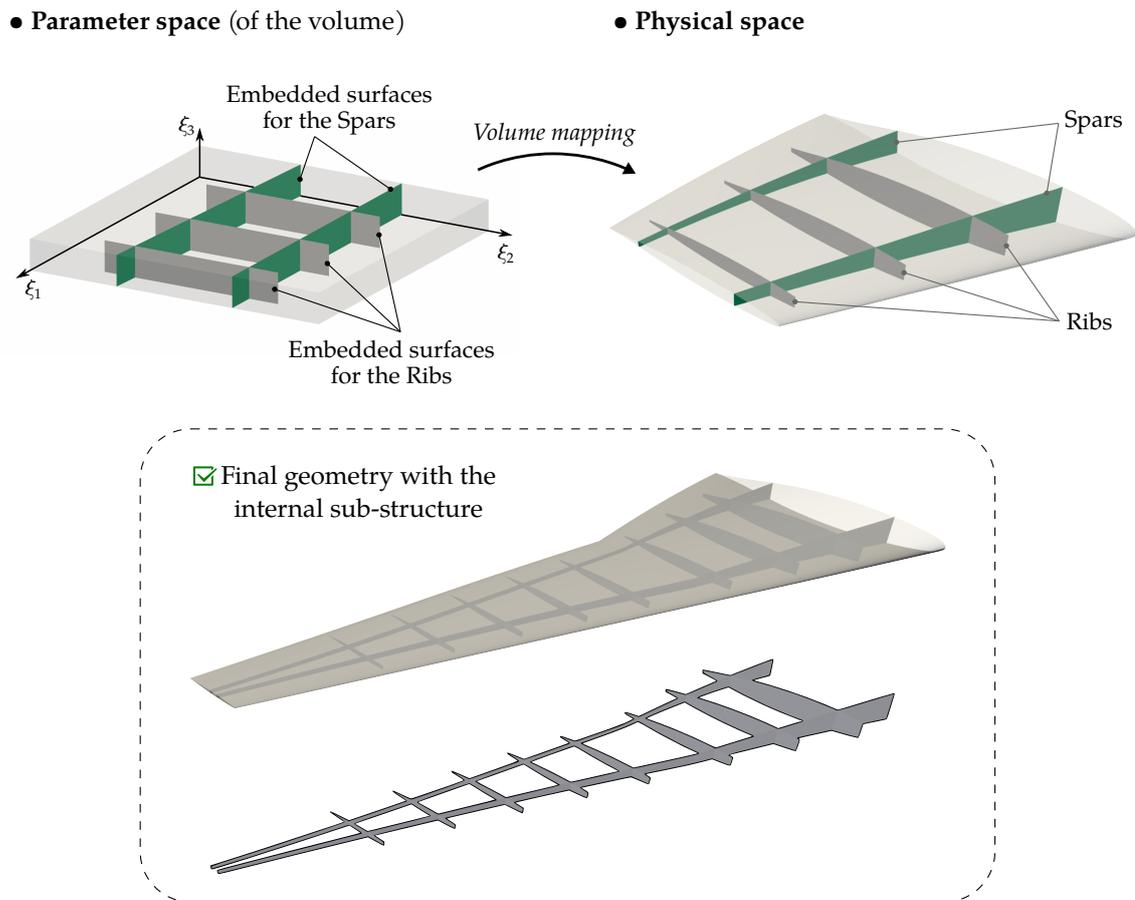
**Figure 6.5** – Geometric modeling of the internal substructure: the spars and the ribs are defined by embedding NURBS surfaces into the parameter space of the previously generated internal volumes (see figure 6.4).
