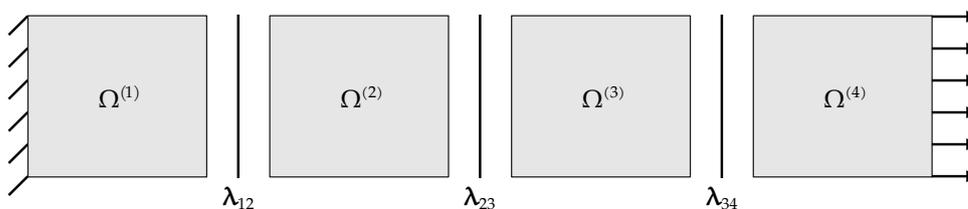
**Figure 4.11** – Parallel computing: the communication between the sub-domains is done through the Lagrange multipliers.
