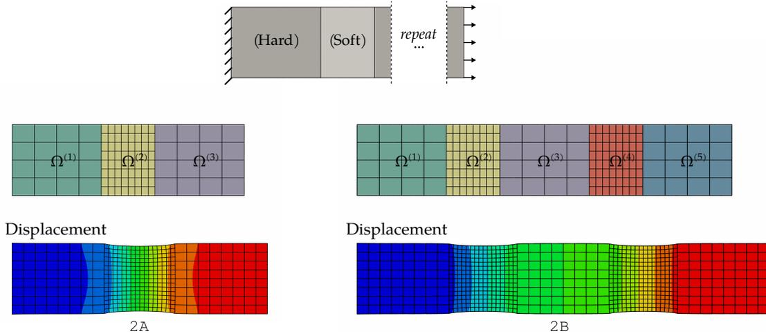
**Figure 4.16** – Description and results of the heterogeneous beam problem. The beam is made of a sequence of hard and soft regions. Configuration 2A has two hard regions separated by one soft region. Configuration 2B has three hard regions separated by two soft regions.
