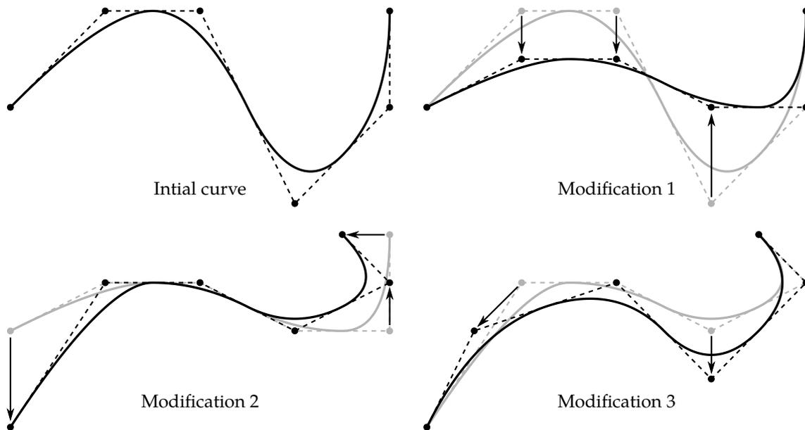
**Figure 2.20** – Example of shape modification by altering the spatial location of the control points.
