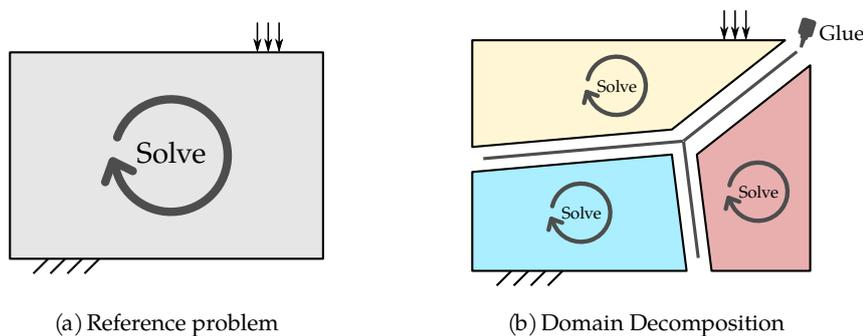
**Figure 4.4** – Non-overlapping Domain Decomposition Methods: (a) instead of solving one large system defined over the whole the computational domain  $\Omega$ , (b) the domain is subdivided into multiple sub-domains  $\Omega^{(s)}$ . The resolution is performed by solving local systems defined per sub-domain, and interface condition are recovered through an iterative process.
