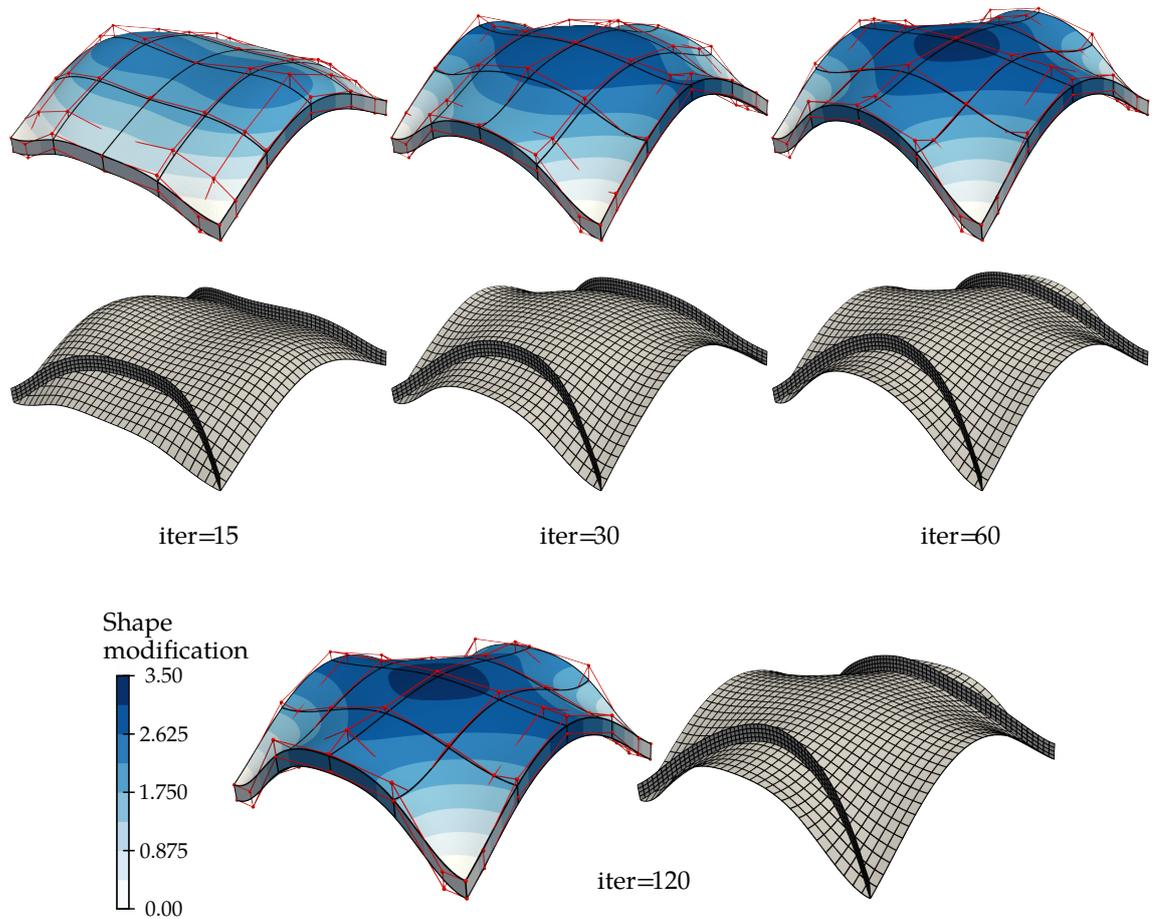
**Figure 6.9** – Several intermediary shapes obtained during the optimization of the stiffened roof.
