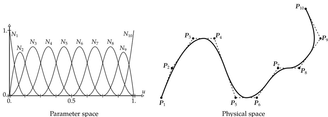
Figure 2.11 – A quadratic B-Spline curve on  $U = \{0, 0, 0, \frac{1}{8}, \frac{2}{8}, \dots, \frac{7}{8}, 1, 1, 1\}$ .
