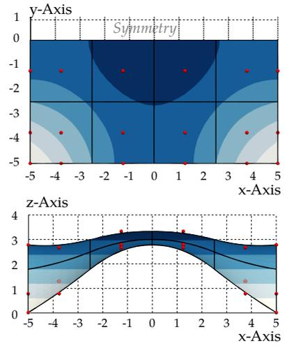
**Step 2. Detailed thickness optimization using solid-shell**
