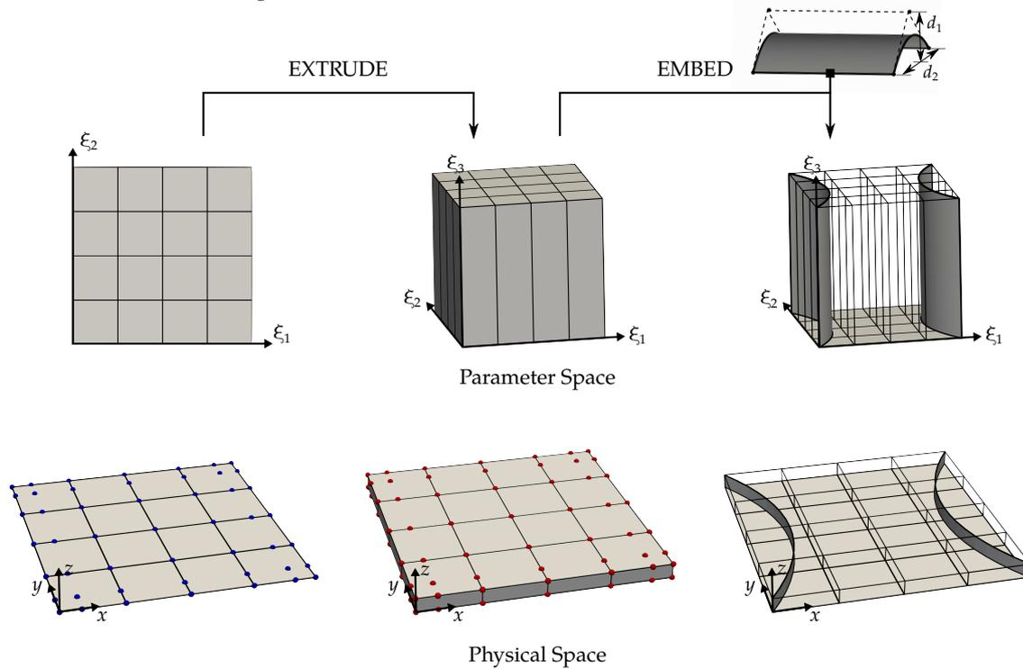
**Figure 6.8** – Settings of the stiffened roof problem. The geometric modeling employs the embedded approach: a volume is extruded from a square plate, and then, the stiffeners are generated by embedding surfaces into the parameter space of this volume.
