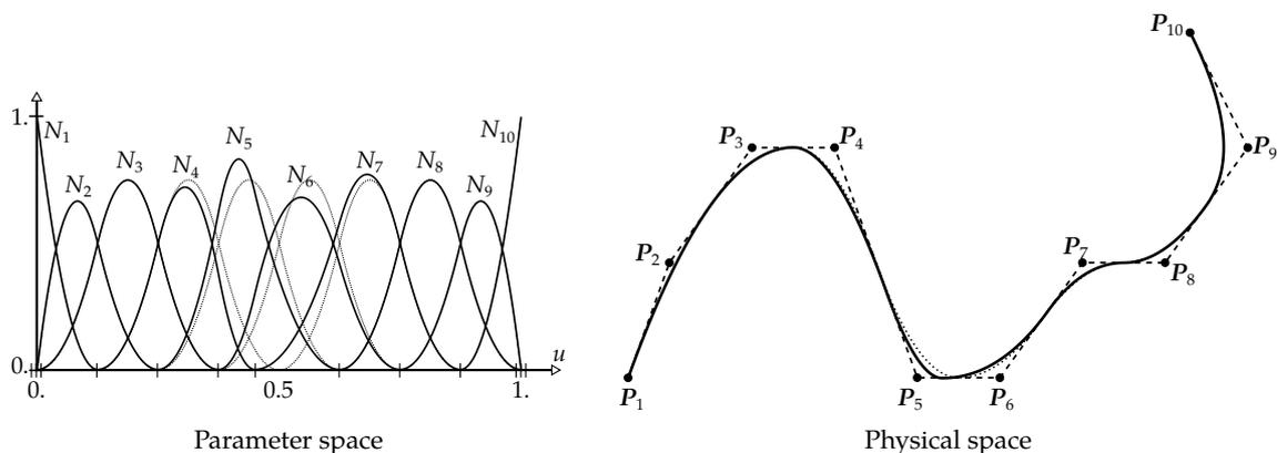
Figure 2.12 – A quadratic B-Spline curve on a non-uniform knot vector. The initial knot  $u_4 = \frac{4}{8}$  used in figure 2.11 has been changed by  $u_4 = \frac{9}{20}$  (the dotted lines repeat the uniform case).
