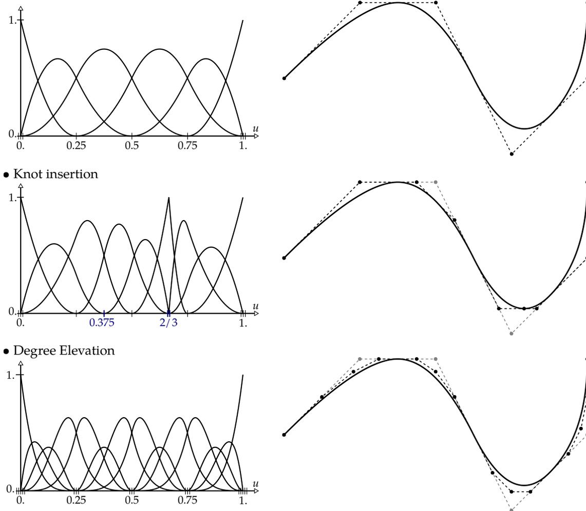
Figure 2.19 – Refinement procedures apply to a B-Spline curve.
