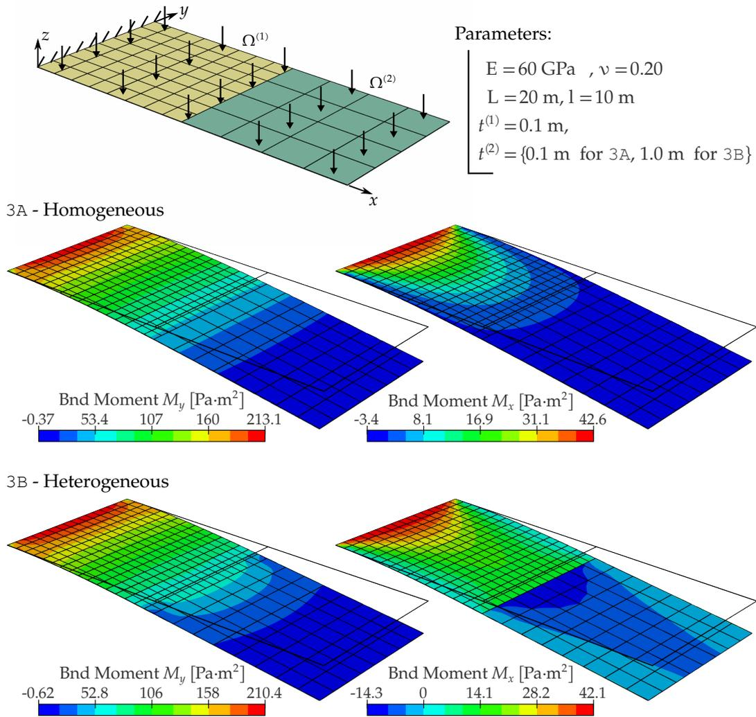
**Figure 4.18** – Description and results of the bending plate problem. The plate is decomposed into two non-matching patches. Two cases are studied: 3A the homogeneous case where the patches have the same properties, and 3B the heterogeneous case where the shells have different thicknesses.
