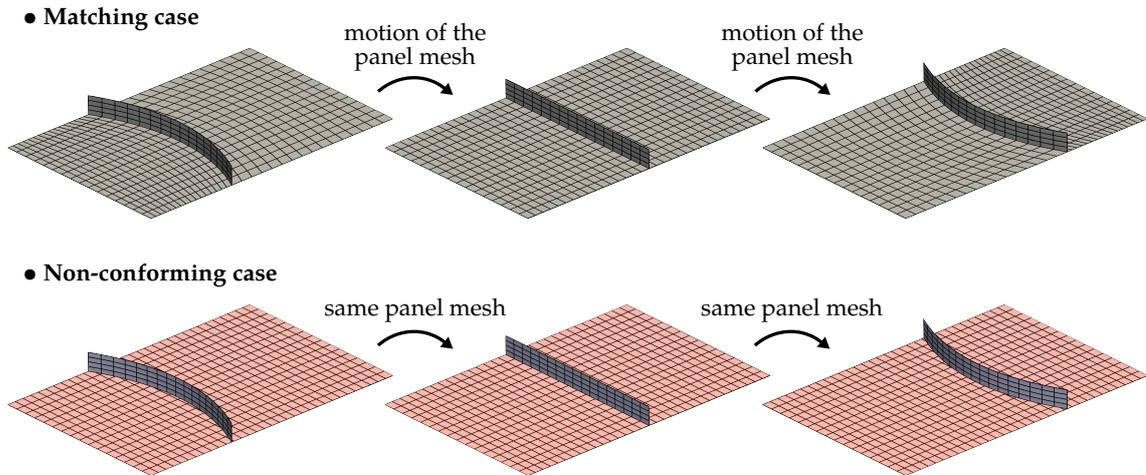
**Figure 6.2** – The discretization of the panel need to be update at each shape modification of the stiffener when a matching multipatch model is used. Using model with non-conforming discretization enables to keep the mesh of the panel untouched.
