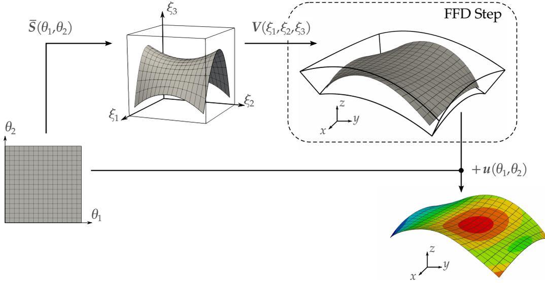
**Figure 5.7** – Overview of the embedded isogeometric Kirchhoff–Love shell elements. The displacement field is approximated by the same parametrization as the embedded surface. However, the embedded surface does not describe the geometry of the shell. An additional mapping step further modifies the geometry of the shell.
