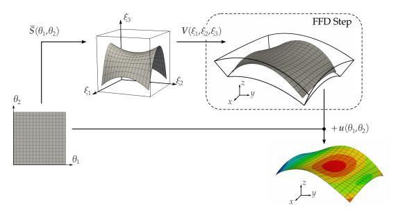
**Figure 5.7** – Overview of the embedded isogeometric Kirchhoff–Love shell elements. The displacement field is approximated by the same parametrization as the embedded surface. However, the embedded surface does not describe the geometry of the shell. An additional mapping step further modifies the geometry of the shell.
