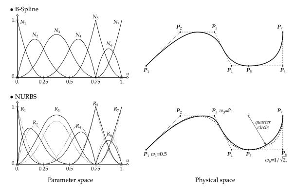
**Figure 2.15** – An example of a NURBS curve: influence of the weights on the basis functions and on the final curve with comparison to the B-Spline case.
