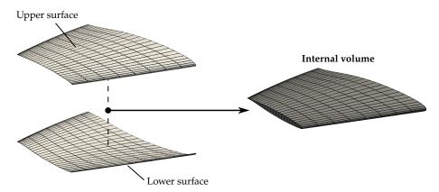
**Figure 6.4** – The upper surface and the lower surface are used to generate a volume that fills the domain delimited by the skin of the wing.
