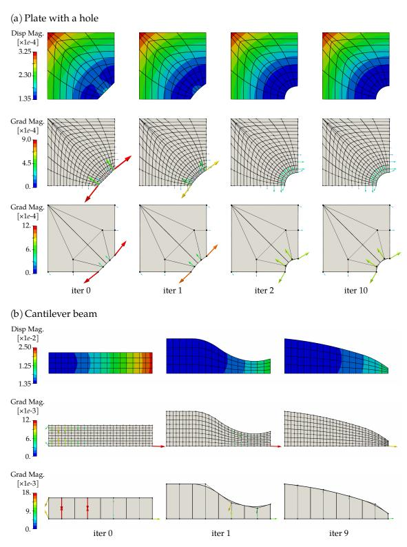
**Figure 3.14** – History of structural analysis and sensitivity analysis during optimization of (a) the plate with a hole (see figure 3.10), and (b) the cantilever beam (see figure 3.12).
