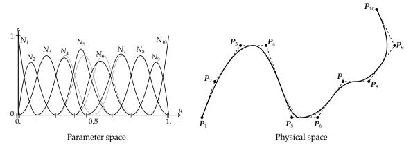
**Figure 2.12** – A quadratic B-Spline curve on a non-uniform knot vector. The initial knot  $u_4 = \frac{4}{8}$  used in figure 2.11 has been changed by  $u_4 = \frac{9}{20}$  (the dotted lines repeat the uniform case).
