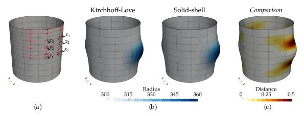
**Figure 3.21** – Shape optimization of the pinched cylinder: (a) 6 design variables update the optimization model, (b) final shapes obtained by both shell formulations, and (c) comparison of the final shapes depicted as the distance between their mid-surface.
