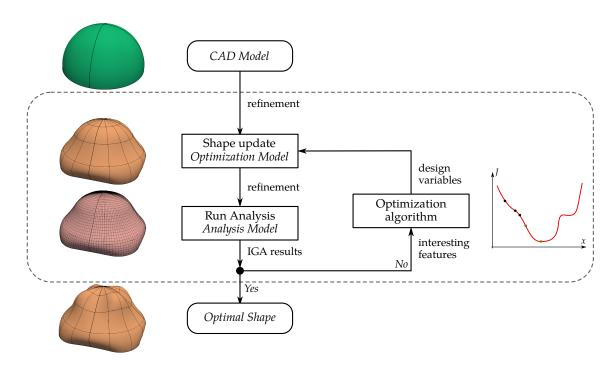
Figure 2.21 – Isogeometric shape optimization flowchart: overview of the main steps.
