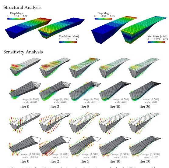
Figure 3.16 – Sensitivity analysis and optimization results for the 3D beam problem.
