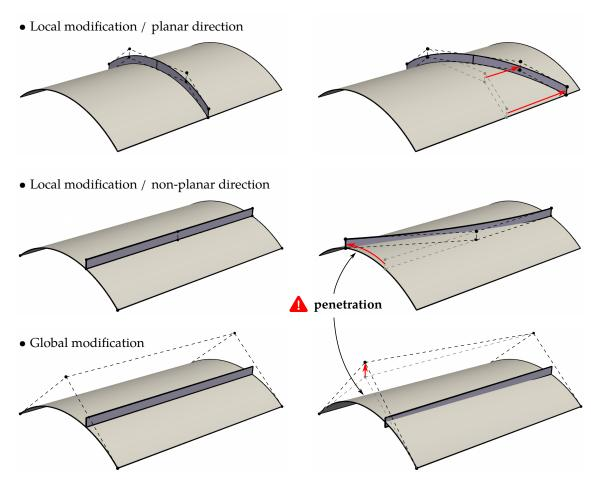
**Figure 5.2** – Moving a stiffener lying on a portion of cylinder. Imposing the shape update in non-planar directions is challenging due to the violation of the bonding condition.
