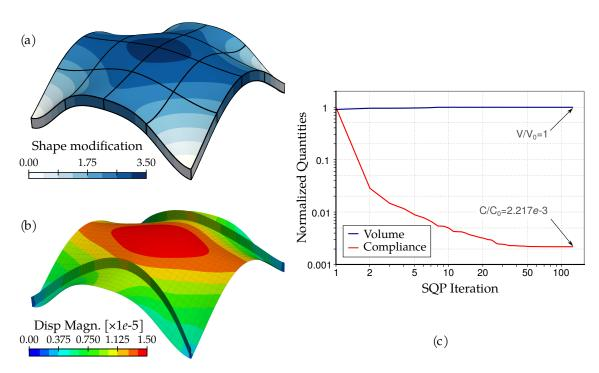
**Figure 6.10** – Final design and result for the stiffened roof problem once the algorithm has converged. The optimal design is much more stiffer than the initial one.
