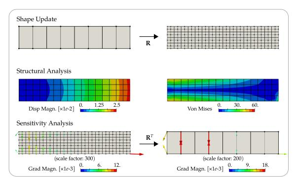
Figure 3.12 – Settings and optimization results for the cantilever beam problem.
