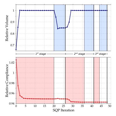
**Figure 3.26** – Optimization history of the bi-step approach applied to the stiffened cylinder problem. Three global iterations with successive shape and sizing steps are preformed until convergence. Red zones denote the shape steps where the compliance is minimized and blue zones denote the sizing step where the volume is minimized.
