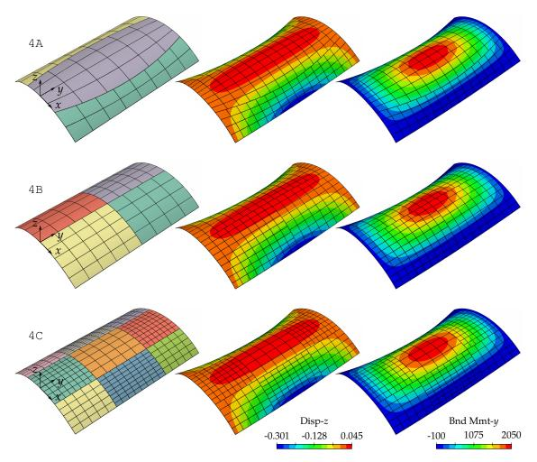
**Figure 4.19** – Description and results for the Scordelis–Lo roof test case. Three different non-matching decomposition are studied: 4A is made of three patches with curved interfaces, 4B is made of four quasi-identical patches (two patches have one more element per direction), and 4C is made of nine patches with different levels of refinement and degrees. (Note: The displacement has unit of length and the bending moment has unit of moment per unit length, respectively).
