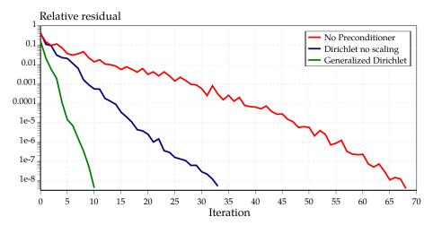
**Figure 4.17** – Convergence of the dual DD solver when applied to the heterogeneous beam problem with five sub-domains 2A (refinement level 4 according to table 4.3). The scaling step of the generalized Dirichlet preconditioner improves drastically the convergence rate.
