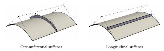
Figure 5.1 – Designing simple stiffeners lying on a portion of cylinder.
