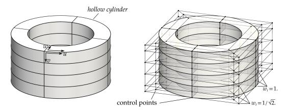
Figure 2.18 – Example of a hollow cylinder described with a quadratic NURBS volume.
