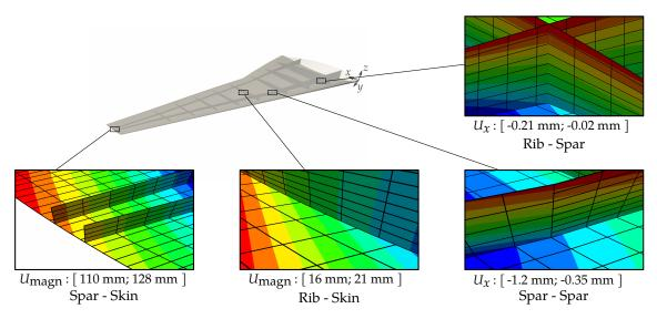
Figure 6.7 – Structural analysis of the CRM wing.
