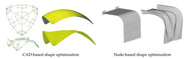
Figure 2.5 – Examples of CAD-based and node-based shape optimization as found in [36].
