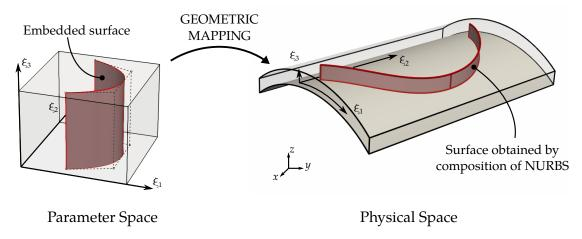
**Figure 5.3** – Construction of a stiffened structure using embedded surfaces. The final surface describing the stiffener is obtained by the composition of a NURBS surface and a NURBS volume. This construction ensures that the stiffener is perfectly lying on the portion of cylinder.
