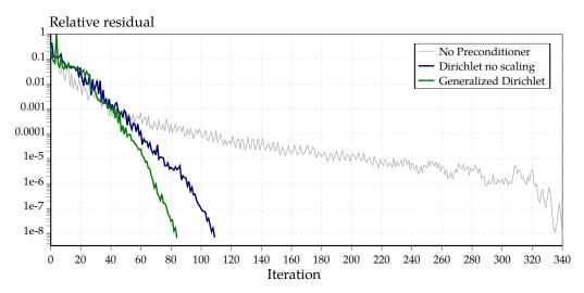
**Figure 4.21** – Convergence plot of the dual DD solver when applied to the stiffened panel 5A (refinement level 2 according to table 4.6). Without the preconditioning step, the solver faces difficulties to converge. The scaling of the generalized Dirichlet preconditioner accelerates the convergence in comparison with the classical Dirichlet preconditioner.
