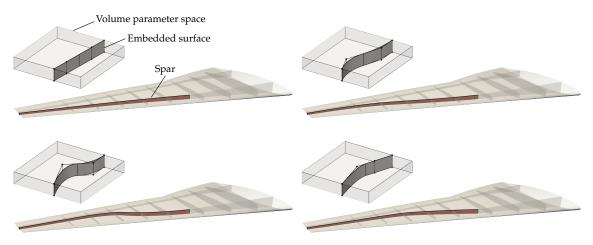
**Figure 6.14** – Shape parametrization of the internal sub-structure of the wing. The shape modifications of the ribs and spars are done by moving the control points of the embedded surfaces.
