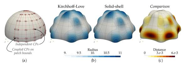
**Figure 3.22** – Shape optimization of the pinched hemisphere: (a) 25 design variables update the optimization model, (b) final shapes obtained by both shell formulations, and (c) comparison of the final shapes depicted as the distance between their mid-surface.
