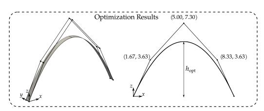
**Figure 3.17** – Settings for the shape optimization of an arch under constant load. The optimal result is a parabola with a specific height to length ratio [72].
