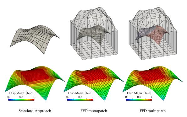
**Figure 5.20** – Comparison of the results obtained for the shape optimization of the square roof. The FFD approach applied to the multipatch model gives very similar results than both monopatch resolutions (standard and FFD).
