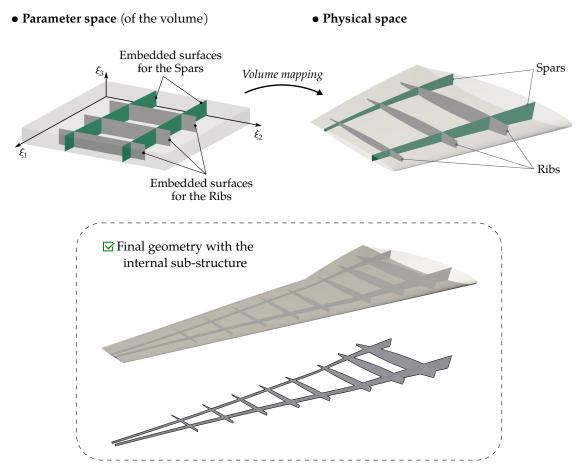
**Figure 6.5** – Geometric modeling of the internal substructure: the spars and the ribs are defined by embedding NURBS surfaces into the parameter space of the previously generated internal volumes (see figure 6.4).
