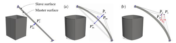
**Figure 3.6** – Definition of the design variables in the context of solid-shell isogeometric elements. (a) A first set of design variables updates the master surface and (b) the slave surface follows the shape variation through a second set of variables.
