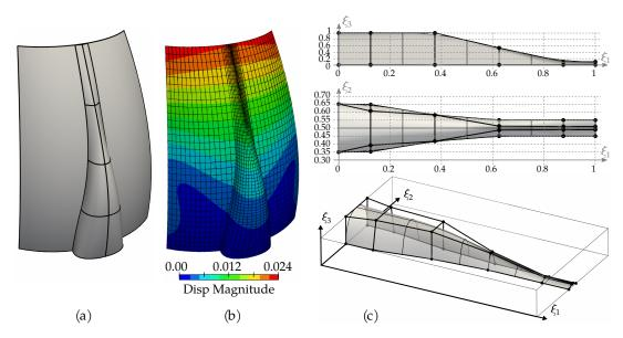
**Figure 6.13** – Optimal configuration of the stiffened curved wall: (a) final geometry and (b) the magnitude of the displacement. (c) The final embedded surface: side, top views and 3D views. The 2D views give information on the coordinates of the control points.
