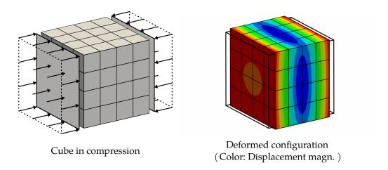
**Figure 4.13** – Pure neumann problem: cube in compression with Poisson's ratio  $\nu = 0.30$ .
