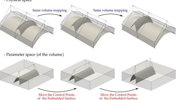
**Figure 5.5** – Using NURBS compositions offers two possibilities for imposing shape deformations. By modifying the volume, one can act on the global shape. By acting on the embedded entities, one can modifying specific parts, as for instance the stiffeners. The bonding condition at the interfaces are automatically satisfied.
