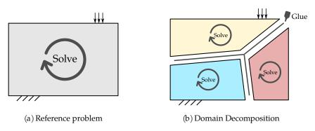
**Figure 4.4** – Non-overlapping Domain Decomposition Methods: (a) instead of solving one large system defined over the whole the computational domain  $\Omega$ , (b) the domain is subdivided into multiple sub-domains  $\Omega^{(s)}$ . The resolution is performed by solving local systems defined per sub-domain, and interface condition are recovered through an iterative process.
