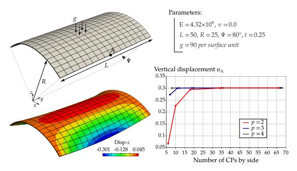
**Figure 3.5** – Scordelis-Lo roof benchmark problem: performance study for the standard solid-shell element.
