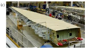
**Figure 1.1** – Stiffened structures are omnipresent in aeronautics: the fuselage (photo (a) from [1] and photo (b) from [2]) and the wing (photo (c) from [3]) are built with this principle.
