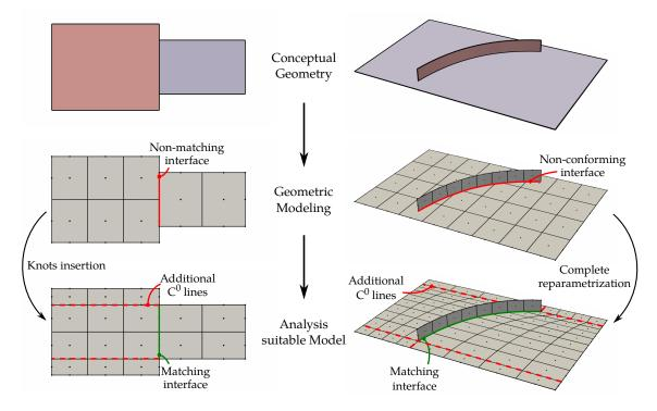
**Figure 4.1** – NURBS modeling generates multipatch geometries where each patch represents a specific part of the complete structure. Naturally, these patches present non-matching or even non-conforming parametrization at their interfaces. Additional procedures are required to get a final model with conforming and matching interfaces.
