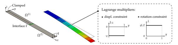
**Figure 4.7** – Cantilever beam with end load: the beam is decomposed in two non-matching pacthes and coupled with the Mortar approach. The shape of Lagrange multipliers for the displacement and the rotation continuity constraints are shown one the right.
