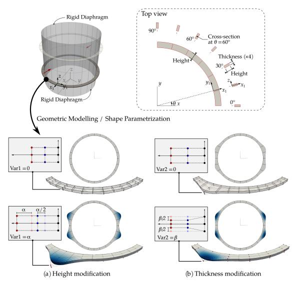
**Figure 3.24** – The stiffened cylinder: two stiffeners are added to the initial pinched cylinder test case. The cross-section of the stiffener can be geometrically parametrized and thus optimized. Here, for each section of control points, two variables impose local design modifications in (a) the height and in (b) the thickness directions respectively.
