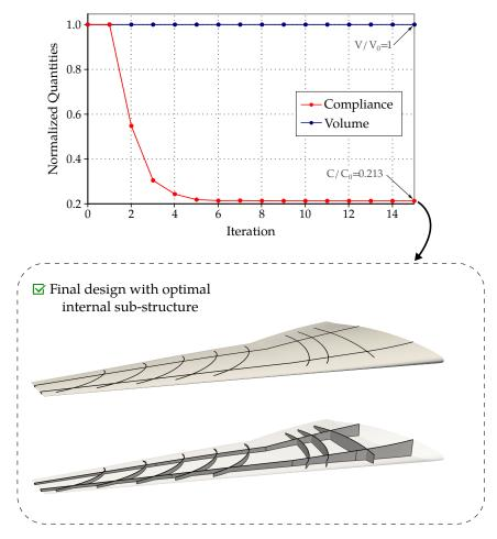
**Figure 6.17** – Optimization histories for the resolution of the wing problem, and final design of the ribs and spars.
