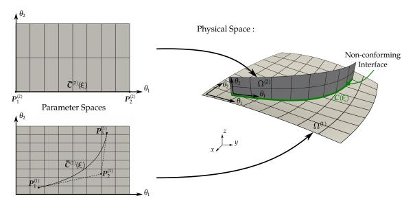
**Figure 4.6** – Non-conforming parametrization: the interface between both surfaces is represented in their parameter spaces by using NURBS curves  $\bar{C}^{(s)}$ . These curves are generated in order to ease the building of the coupling operators for the Mortar approach.
