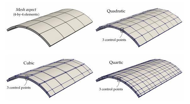
**Figure 3.4** – Discretization with the isogeometric standard solid-shell element. Degree 2 is always chosen through the thickness, no matter the degree in the two principal directions.
