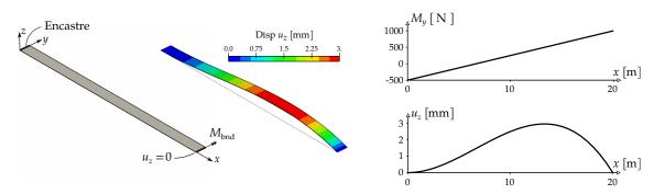
**Figure 4.10** – Beam with one end fixed and a bending moment applied on the other edge. The bending moment can be applied using the Mortar operator **Z**.
