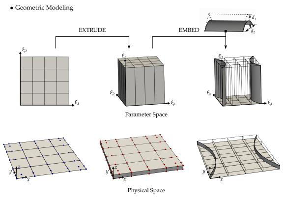
**Figure 6.8** – Settings of the stiffened roof problem. The geometric modeling employs the embedded approach: a volume is extruded from a square plate, and then, the stiffener are generated by embedding surfaces into the parameter space of this volume.
