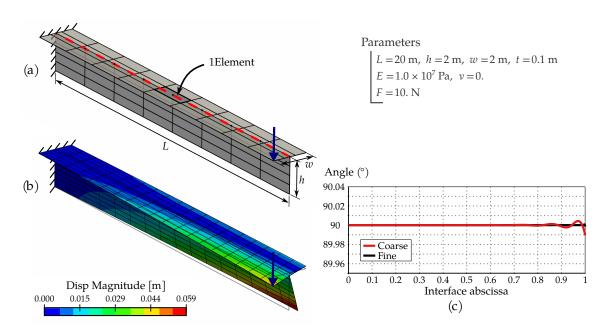
**Figure 4.8** – T-Beam non-matching coupling: (a) Description of the problem: the interface cuts the upper patch at the middle of some elements. (b) Deformed configuration with scale factor of 10 and the magnitude of the displacement field. (c) Angle between the patches along the interface after deformation. Coarse case corresponds to the mesh depicted in (b). Fine mesh is three times refined.
