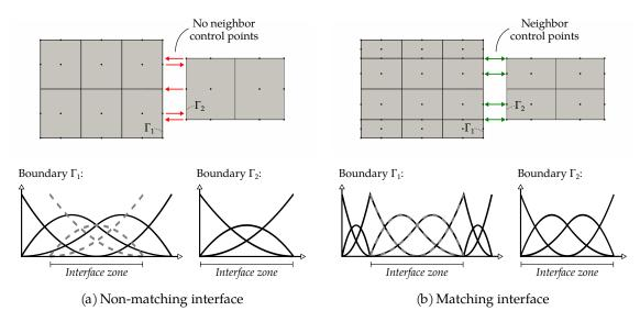
**Figure 4.2** – Connecting conforming patches that are initially non-matching (a): the basis functions of both patches need to be modified in order to become identical over the interface zone (b).
