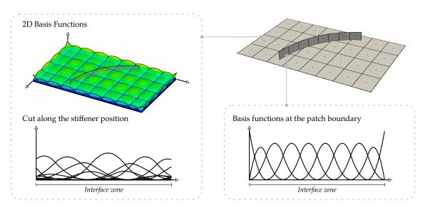
**Figure 4.3** – Example of a stiffened panel with non-conforming parametrizations: the interface crosses the elements from the panel. The trace spaces of both sides are particularly different.
