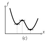
**Figure 3.2** – Recognizing a minimizer of a smooth function: (a) the first derivative equals to zero at the global minimum, but this condition is not sufficient to identify the global minimizer as highlight in cases (b) and (c).
