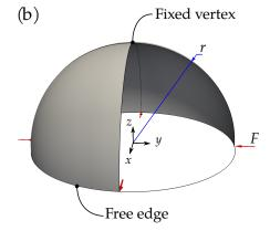
**Figure 3.20** – Numerical examples to investigate the use of isogeometric solid-shell elements for shape optimization of shell structures: (a) pinched cylinder and (b) pinched hemisphere.
