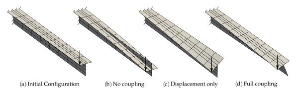
**Figure 4.5** – Kinematic constraints for Kirchhoff–Love shells: at the patch junction, the three components of the displacement fields need to be coupled (c). Additionally, the continuity of the rotation in the tangent direction of this interface curve is imposed (d).
