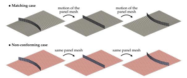
**Figure 6.2** – The discretization of the panel need to be update at each shape modification of the stiffener when a matching multipatch model is used. Using model with non-conforming discretization enables to keep the mesh of the panel untouched.
