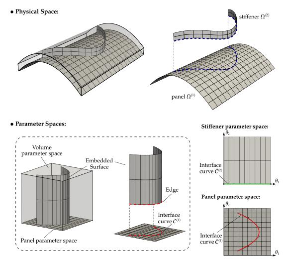
**Figure 5.13** – Definition of the interface curves with the embedded approach. For the stiffener, the interface curve  $\check{\mathbf{C}}^{(2)}$  lies on one edge of the embedded surface. For the panel, the interface curve  $\check{\mathbf{C}}^{(1)}$  can be extracted from the embedded surface.
