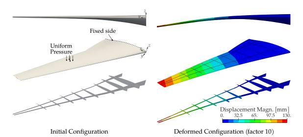
Figure 6.6 – Structural analysis of the CRM wing.
