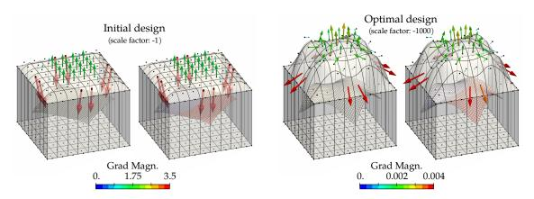
**Figure 5.21** – Comparison of the sensitivity analysis results of the FFD approach when applied to the monopatch or the multipatch model.
