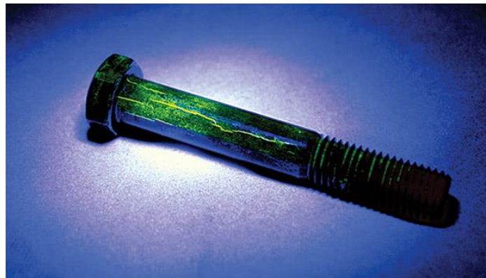
Figure 1.5. A screw inspected using Magnetic Particle Inspection [Magn]
