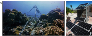
Fig 1. a) Tripod supporting the hydrophone and the waterproof container (data acquisition chain); b) terrestrial interface (power supply, data storage)
