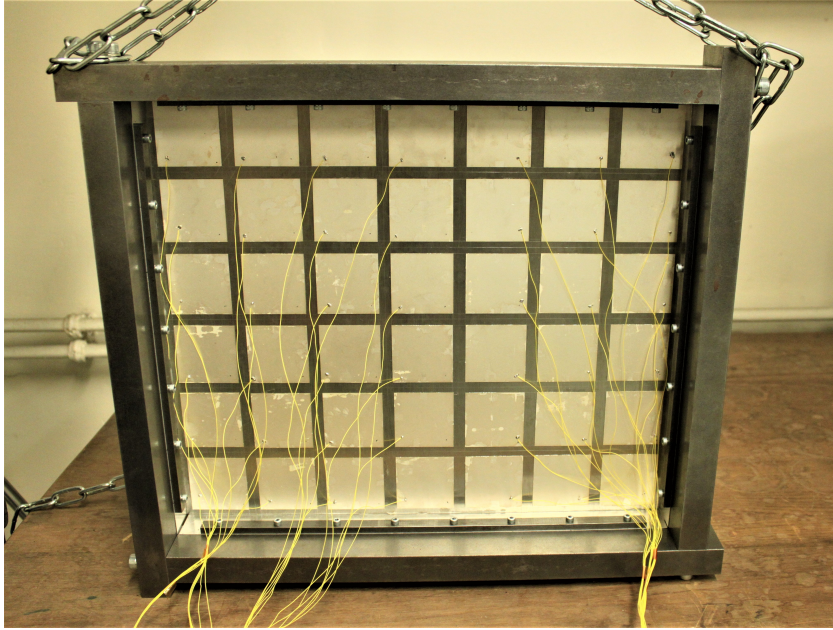
Figure 3.3: Duralumin rectangular plate periodically covered by 42 square piezoelectric patches and simply-supported by a steel frame.
