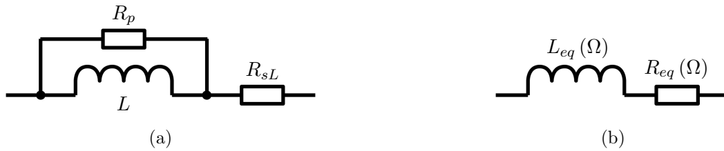
Figure 4.5: (a) Electrical model of a resistive inductor including magnetic losses and (b) equivalent series representation with frequency-dependent lumped elements.
