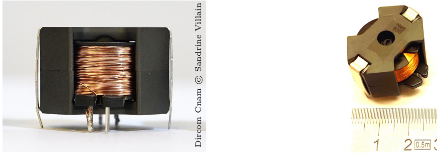
Figure 4.4: Produced fully passive N48-ferrite based inductor with a RM 10 core geometry.
