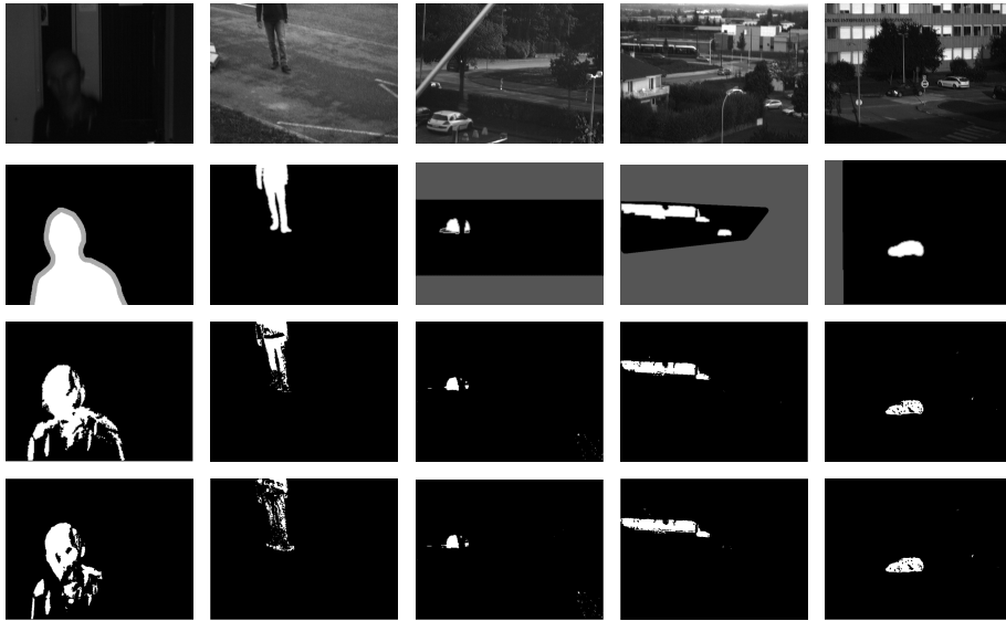
Figure 3.8: Background subtraction results on five videos. The top row is original multispectral sequences, the second row is the corresponding ground truth and the last two rows are the results obtained by the respect best combination of three-channel based multispectral and RGB sequences, respectively.
