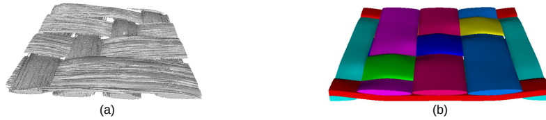
Figure 2.32 – \mu CT reconstruction (a) and TexGen model (b) of a Chomar 4H satin glass fabric [Sherburn2007]
