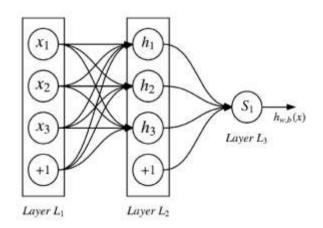
Figure 11 - The structure of a feedforward neural network
