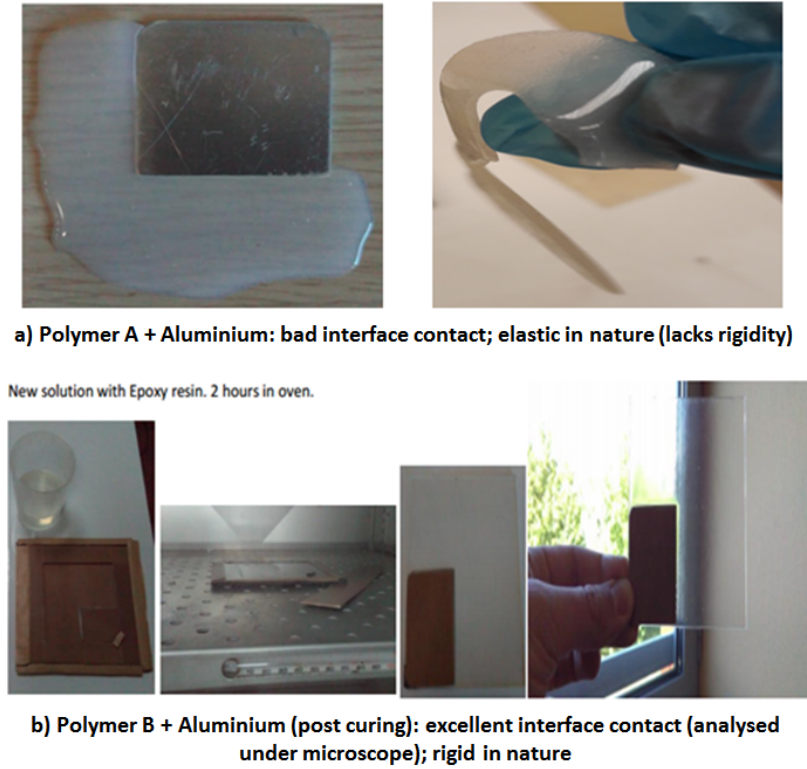
Figure 3: Testing material combinations : a) aluminum with polymer A and b) aluminum with polymer B.
