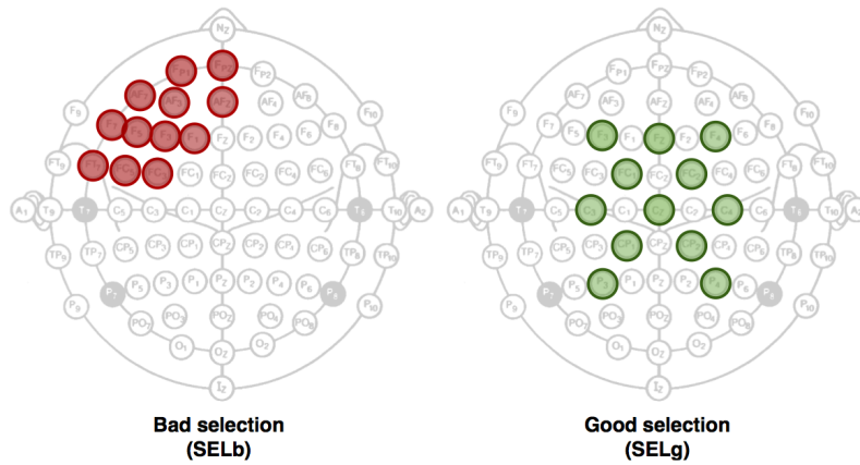
Fig. 3.1: Position of the 12 electrodes selected for the SELb+MDM pipeline (in red) and the SELg+MDM pipeline (in green).
