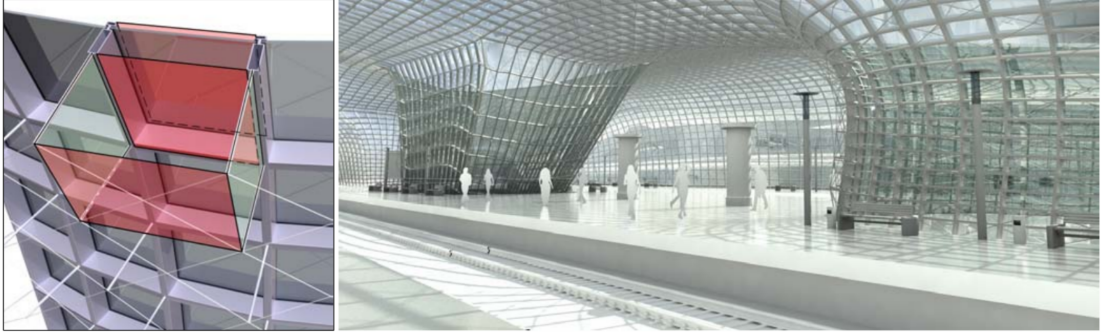
FIGURE 2.4: Architectural design made using subdivision of conical meshes, which is a specific case of PQ meshes. Illustration taken from [LPW + 06].
