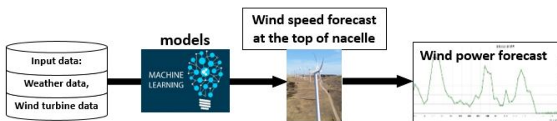
FIGURE 3 – Indirect Approach to wind power forecasting
