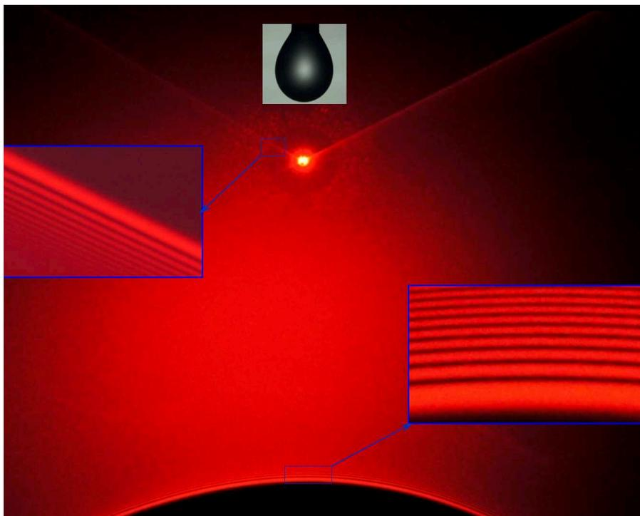
Figure 4.5: Forward scattering pattern of a pendent droplet with a perpendicularly polarized plane wave ( $\lambda = 0.6328 \mu\text{m}$ ). Detection angle in horizontal direction and in vertical direction are both about  $[-30^\circ, 30^\circ]$ .
