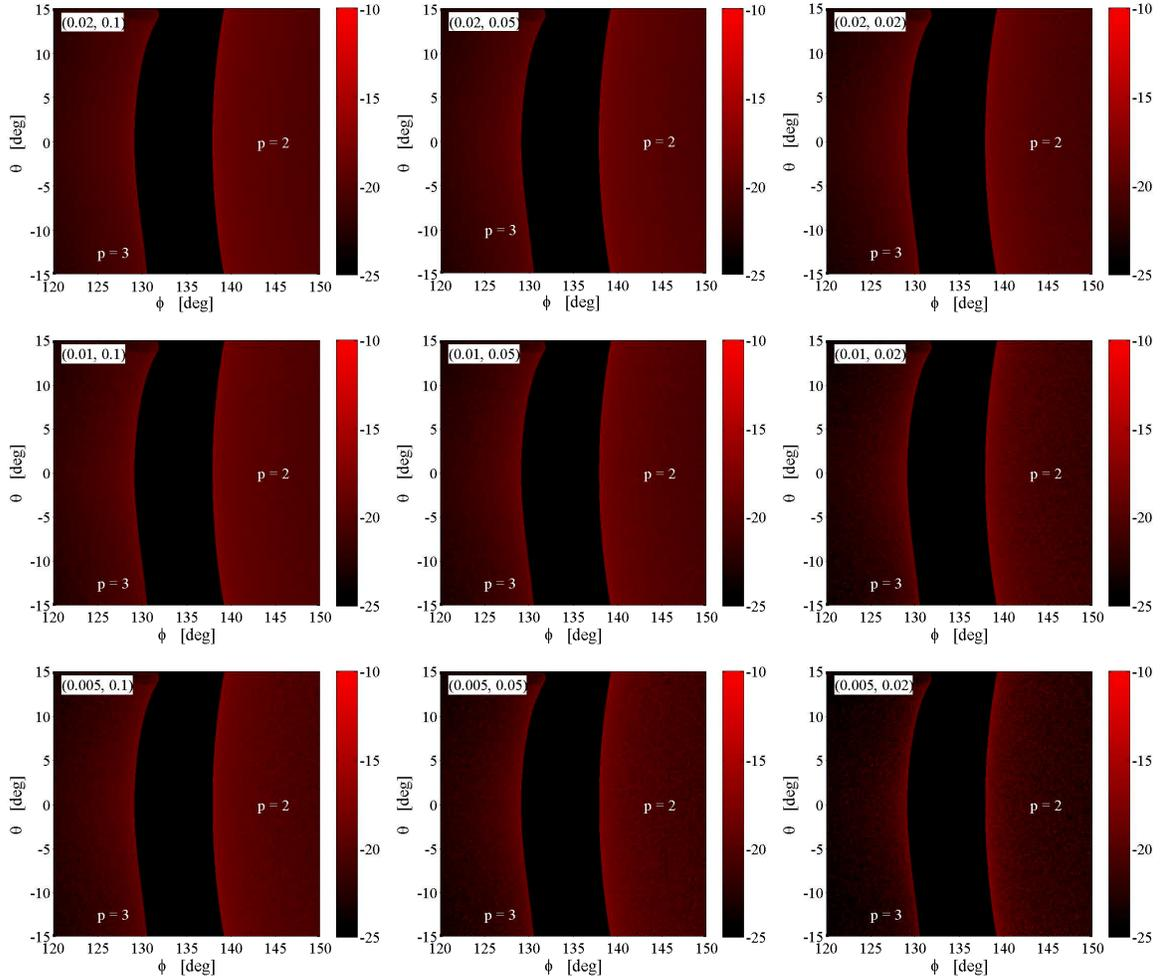
Figure 5.11: Scattering patterns **without interference** of the pendent droplet **a** with parameters given in Tab. 5.4 and  $R_e = 541.15 \mu\text{m}$ ,  $H = 989.86 \mu\text{m}$ . The 9 images correspond to the simulation with 9 pairs of detection steps ( $C_\phi, C_\theta$ ) given in Tab. 5.4
