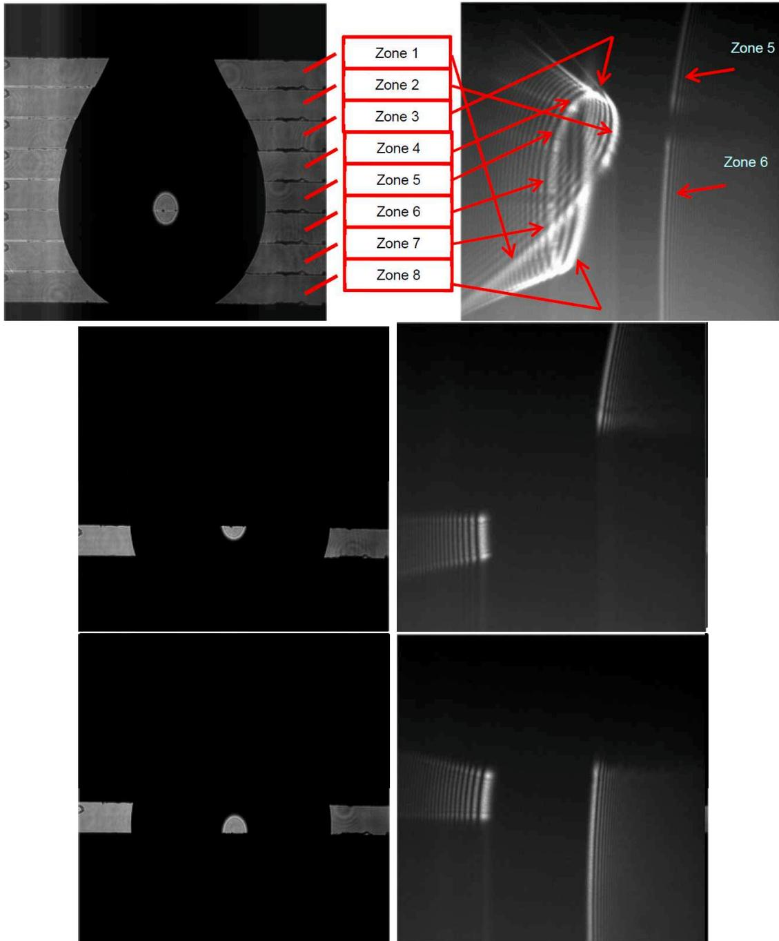
Figure 4.4: Scattering pattern (zones) of a pendent droplet with a perpendicularly polarized plane wave ( $\lambda = 0.6328 \mu\text{m}$ ). Detection angle in horizontal direction is about  $[110^\circ, 150^\circ]$  and that in vertical direction is about  $[-20^\circ, 20^\circ]$ .
