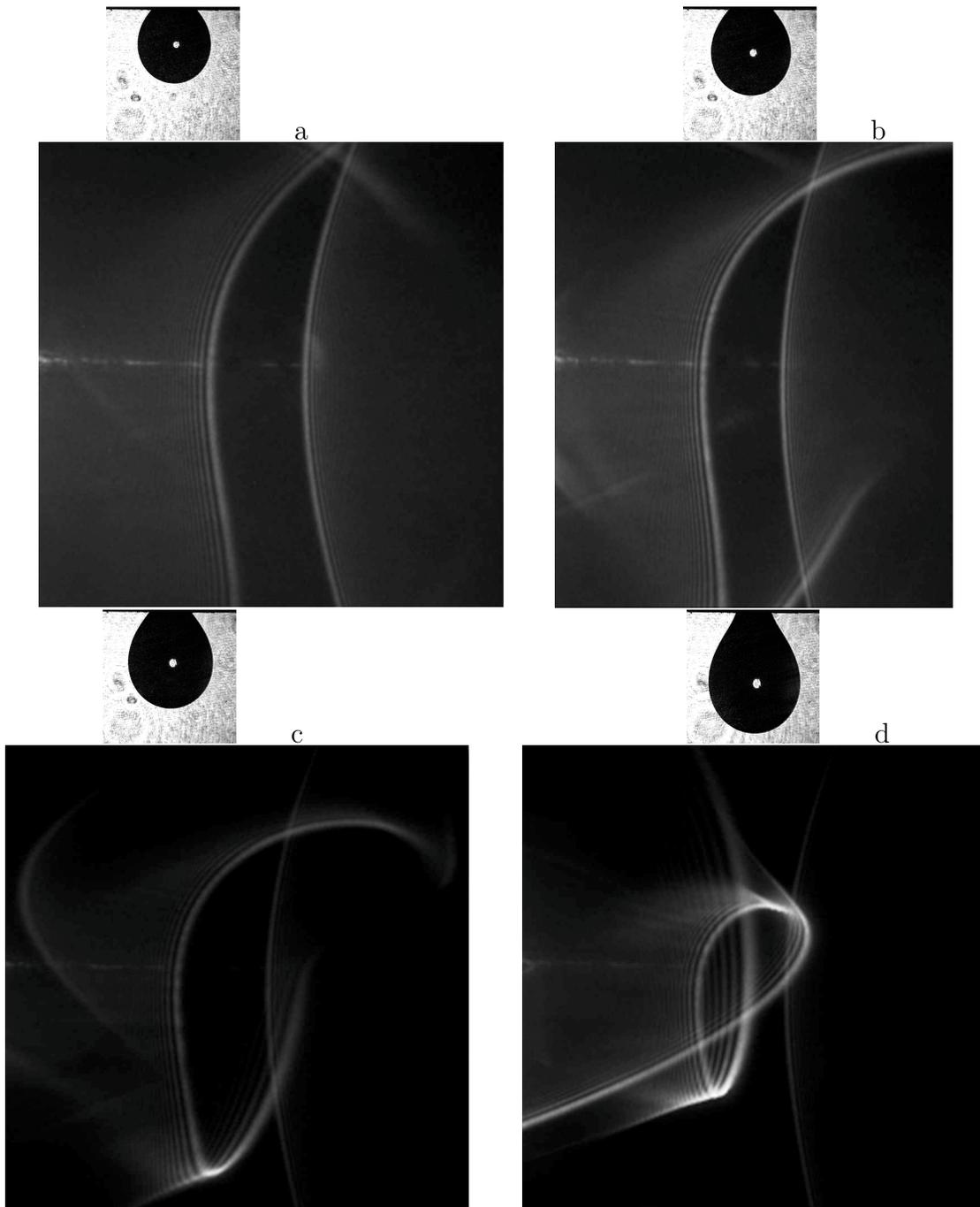
Figure 4.3: Experimental images of four pendent droplets and their scattering patterns around the rainbow angles with a perpendicularly polarized plane wave ( $\lambda = 0.6328 \mu\text{m}$ ). Detection angle in horizontal direction is about  $[70^\circ, 170^\circ]$  and that in vertical direction is about  $[-40^\circ, 40^\circ]$ .
