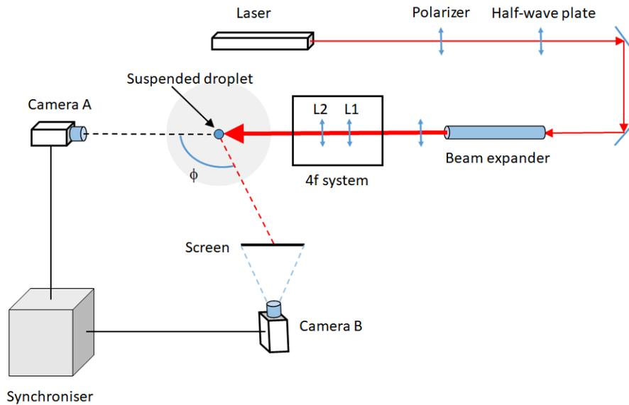
Figure 4.2: Schematic diagram of the experimental setup systems
