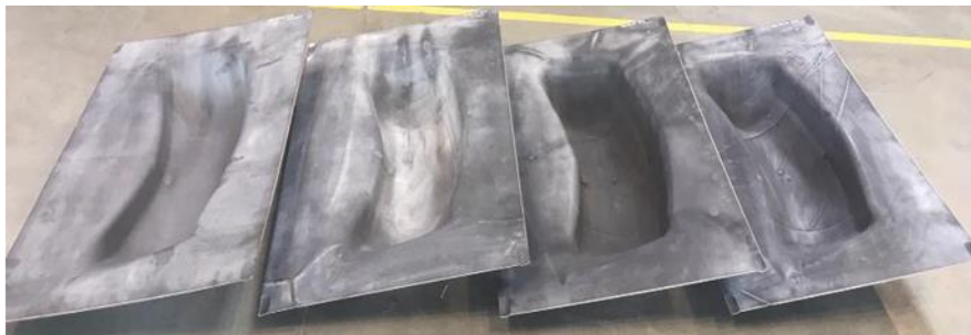
Four consecutive IR formed sheets before chemical milling and final trimming
