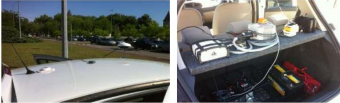
Figure 5-2. Top of the vehicle roof (left) with the Novatel antenna in white and the Ublox antenna in black; Inside the vehicle (right) the Novatel receiver and the inertial unit side-by-side.
