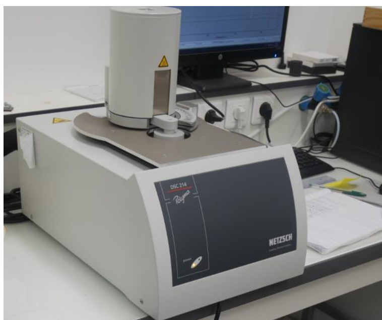
Figure A. I-3: Photography of the DSC apparatus used in this work
