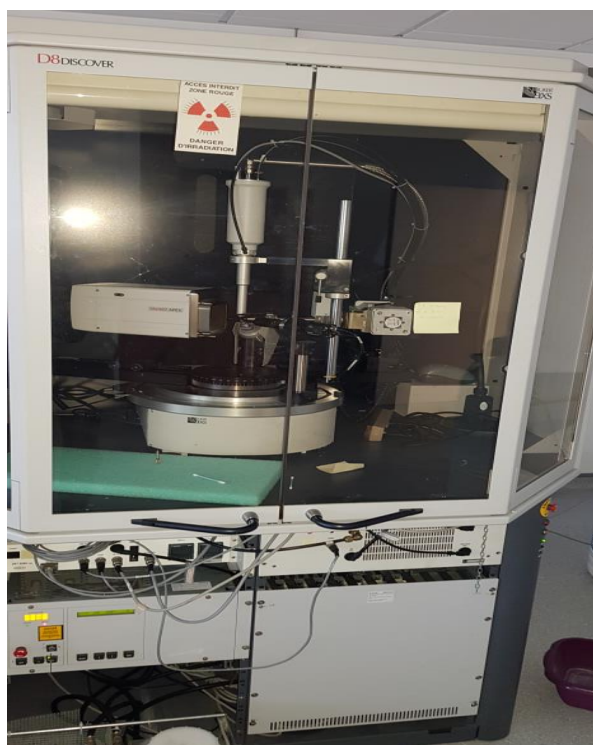
Figure A. I-2: Photography of the SC-XRD used for this work
