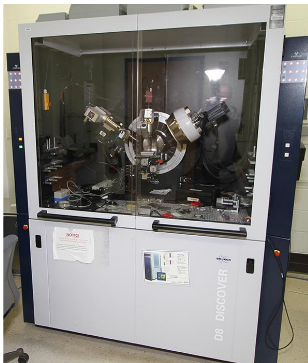
Figure A. I-1: Photography of the XRPD used for this work
