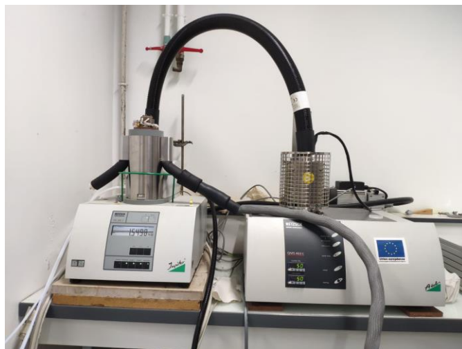
Figure A. I-4: Photography of the TGA-DSC apparatus used in this work
