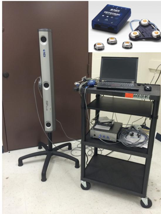
FIGURE 2.11: Optotrak 1D tracking system. Markers for the system shown in top right. (Images from [publish.illinois.edu](http://publish.illinois.edu) and [www.ndigital.com](http://www.ndigital.com))
