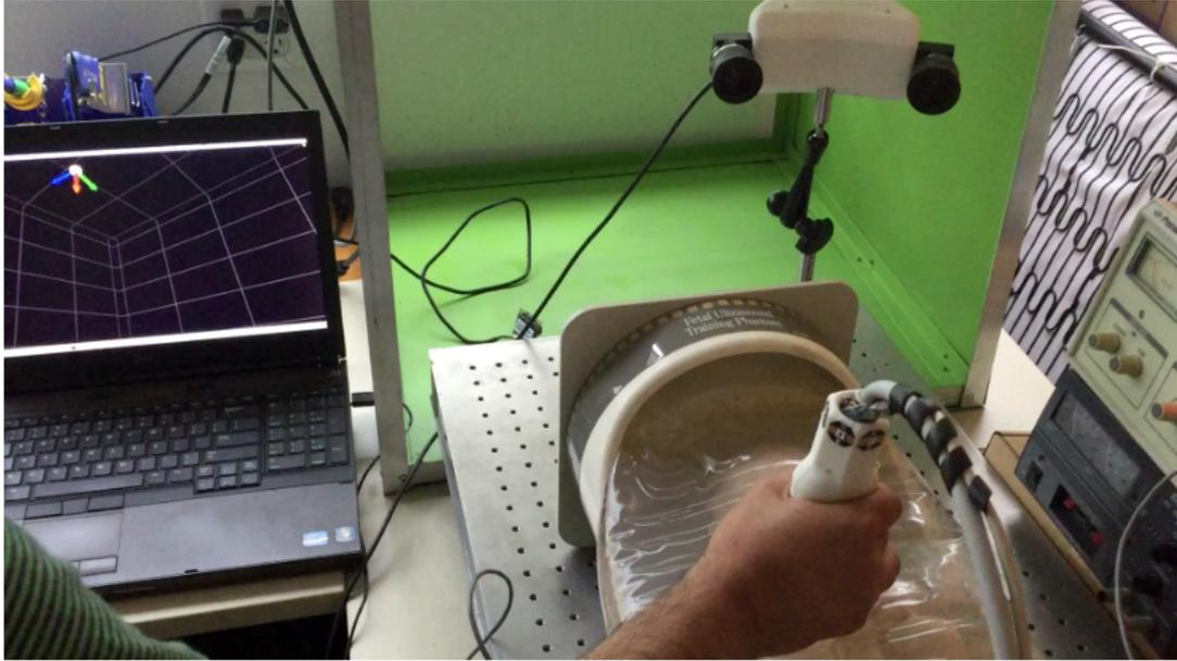
FIGURE 3.6: PSD camera pointing at the LED ring mounted on a US probe handle. (Image from Siemens Healthcare)
