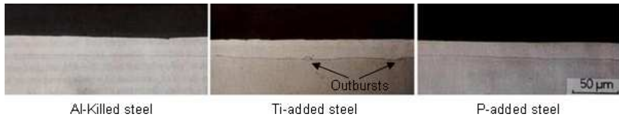
Figure 33: Cross section micrographs showing the effects of the steel chemical composition on the kinetics of the inhibition layer breakdown during galvanizing in a zinc bath containing 0.16 wt.% Al at 450 °C for 15 s (Hisamatsu [25]).
