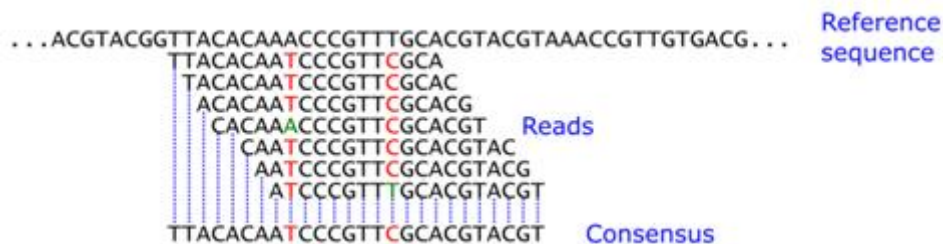
FIGURE 14: COMPARATIVE ASSEMBLY: READS ARE ALIGNED TO A REFERENCE SEQUENCE (ADAPTED FROM WAJID & SERPEDIN, 2016)
