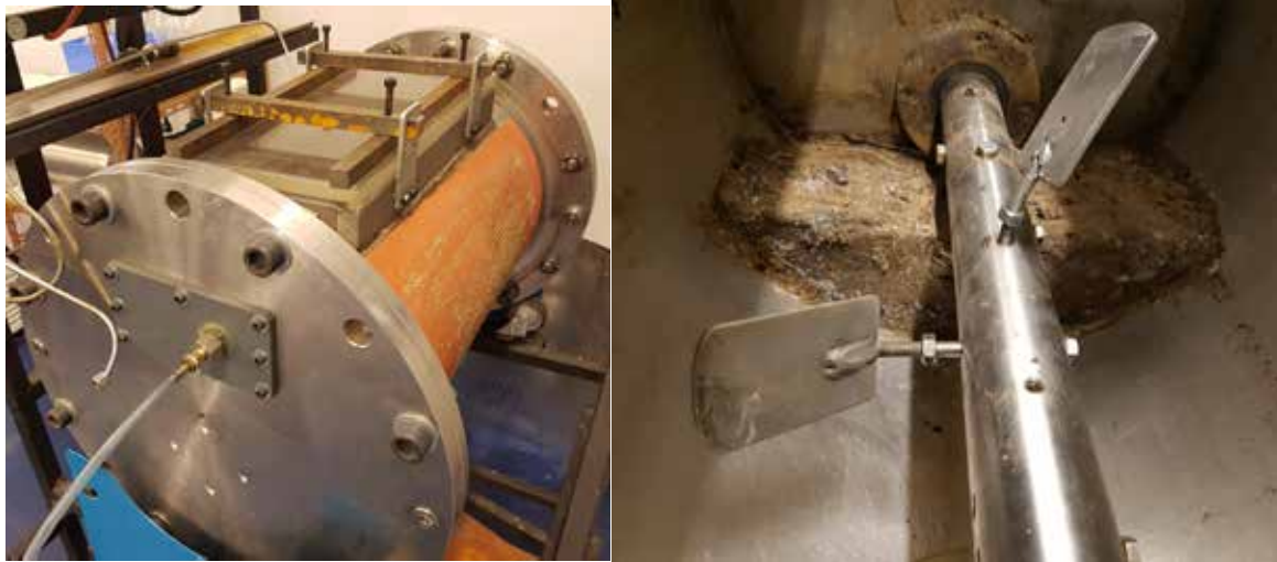
Figure a – On the left, reactor used. On the right, the stirrer in the reactor with a concrete wall in the bottom figuring the average level of reactor content.
