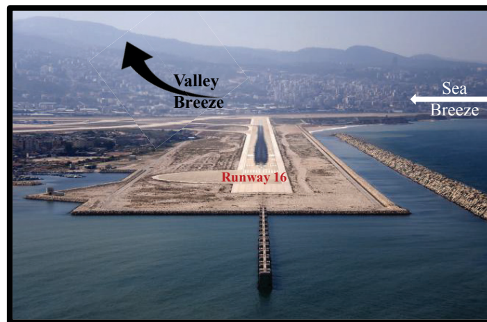
Figure 3-6: The interaction between sea breeze and valley breeze, expected to carry pollutants from Beirut Airport inwards towards the citizens and upslope towards the mountainous areas
