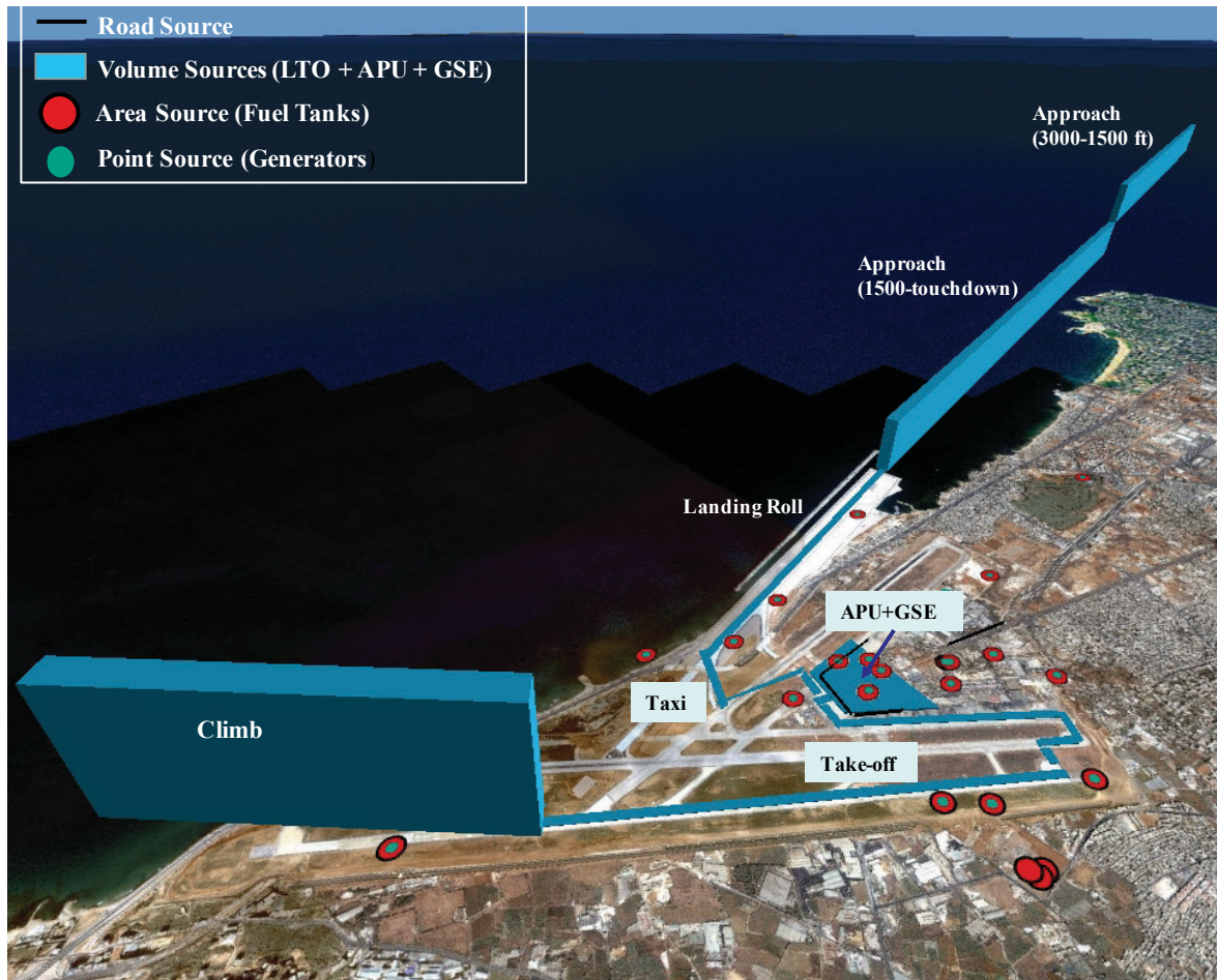
Figure 8-5: 3-D geospatial emissions inventory created by exporting EMIT database to Arc Globe for the sources modelled at Beirut Airport in this study (2012)
