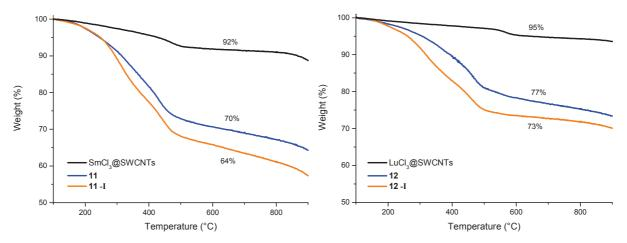
Figure 5.3 TG curves of pristine, amino-functionalized and tag-functionalized SmCl<sub>3</sub>@SWCNTs (left) and LuCl<sub>3</sub>@SWCNTs (right).
