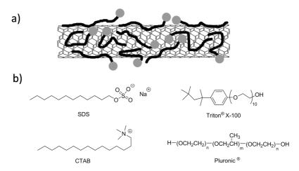
**Figure 1.4** (a) Schematic representation of the random adsorption of surfactant molecules onto the SWCNT sidewalls. (b) Chemical structures of some of the most used surfactants and polymers (SDS: sodium dodecyl sulfate; CTAB: hexadecyltrimethylammonium bromide). Figure adapted from ref. [73].
