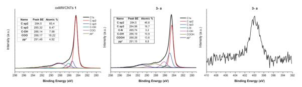
Figure 2.1 XPS spectra: C1s with fitting for oxMWCNTs 1 and aminated MWCNTs 3-a (left and center), N1s for MWCNTs 3-a (right).
