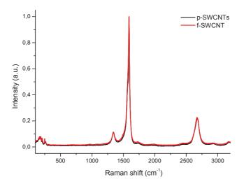
**Figure 5.1** Raman spectra of SWCNTs before (p-SWCNTs) and after (f-SWCNTs) performing Bingel reaction at r.t. The spectra is the average of measurements on two areas, and values were normalized on the G band maximum value. No variation in the intensity of the D band can be noticed.
