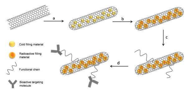
**Figure 4.4** General representation of the procedures for the preparation of f-X@CNTs (X = general metal) for the delivery of radioactivity. a) Filling and sealing of purified CNTs with non-radioactive isotopes, b) irradiation of X@CNTs, c) covalent functionalization, d) conjugation of the bioactive target.
