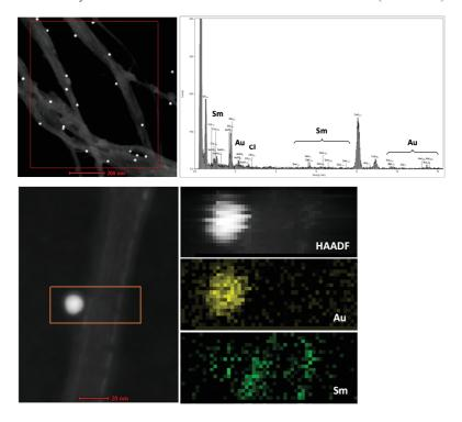
**Figure 5.10** Dark-field STEM images of conjugate **19-Ab** after staining with anti-human IgG/AuNP. (Top) EDX analysis of the area in the red rectangle. (Bottom) STEM HAADF image, Au and Sm mapping of the area in the orange rectangle by EDX. Images and analysis collected by Elzbieta Pach and Dr. B. Ballesteros from ICN 2 (Barcelona).
