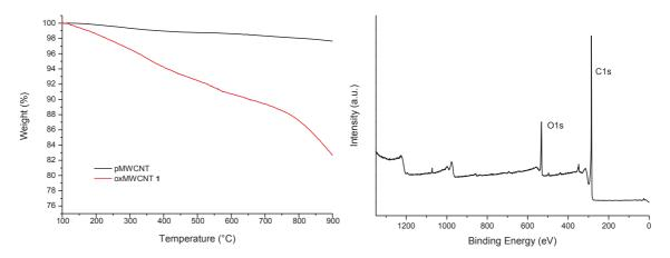
Figure 2.7 Thermogravimetric curves of pMWCNTs and oxMWCNTs 1 (left), and XPS spectrum of oxMWCNTs 1.
