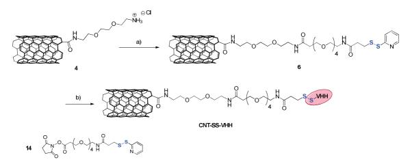
Scheme 3.7 Synthesis of conjugate CNT-SS-VHH: a) 14, DIEA, DMF, r.t., 48 h; b) VHH, EDTA, PBS, r.t., 6 h
