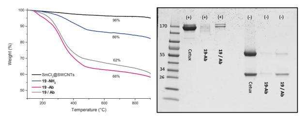
Figure 5.8 (Left) TG curves of pristine SmCl<sub>3</sub>@SWCNTs-B2 and conjugates 19-NH<sub>2</sub>, 19-Ab and 19/Ab. (Right) Gel electrophoresis of Cetuximab, 19-Ab and 19/Ab run under non-reducing (+) and reducing conditions (-) at 150 keV. Gel stained with Coomassie blue. Protein size marker on lane 1 (size in kDa).
