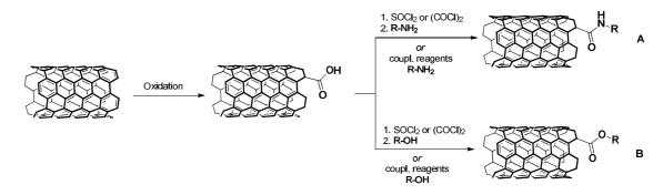
**Scheme 1.1** Oxidation of CNTs followed by activation and amidation (A) or esterification (B). For clarity, a SWCNT fragment is represented with only one single added functional group.
