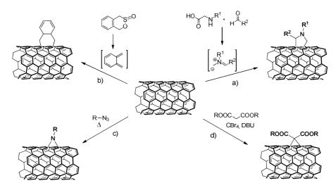
**Scheme 1.2** Examples of cycloaddition reactions on CNTs: a) 1,3-dipolar cycloaddition, b) Diels-Alder reaction, c) nitrene and d) Bingel reaction.
