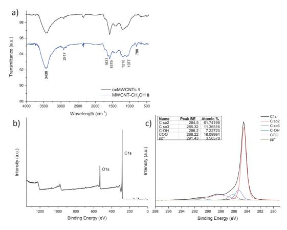
Figure 2.10 Characterization of compound 8. FT-IR (a) and XPS spectra: general survey (b), C1s (c).
