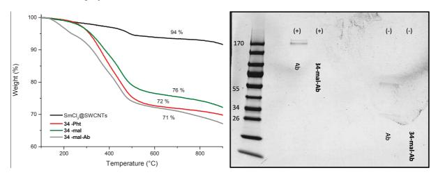
Figure 5.7 (Left) TG curves of pristine SmCl<sub>3</sub>@SWCNT-B3 and conjugates 34-Pht, 34-mal and 34-mal-Ab. (Right) Gel electrophoresis of Cetuximab and 34-mal-Ab run under non-reducing (+) and reducing conditions (-) at 150 kV. Gel stained with Coomassie blue. Protein size marker on lane 1 (size in kDa).
