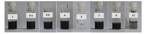
Figure 2.4 Dispersibility of oxMWCNTs and aminated MWCNTs in ddH<sub>2</sub>O at a concentration of 0.2 mg/mL.
