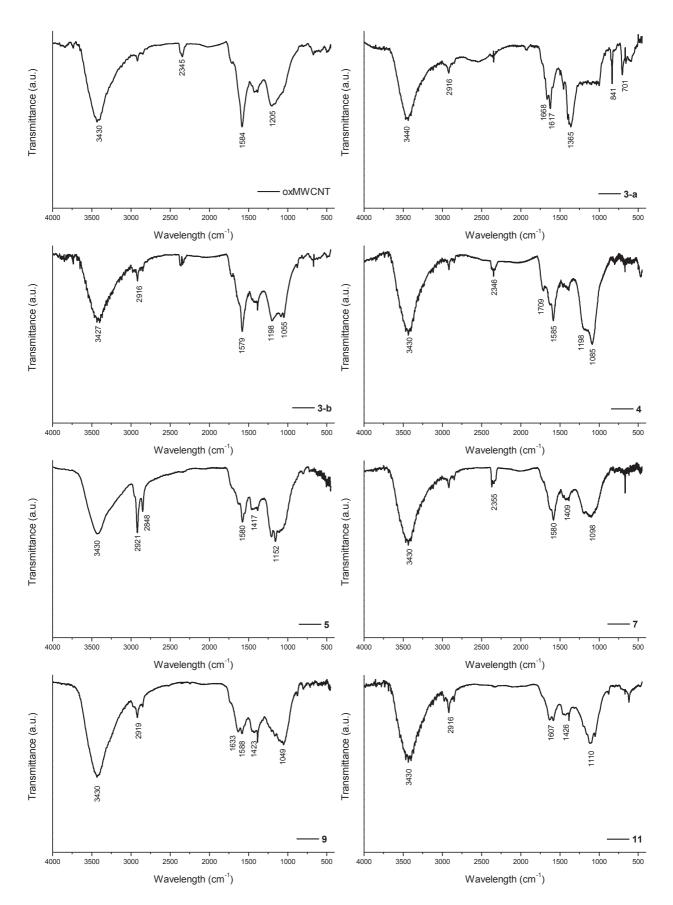
Figure 2.2 FT-IR spectra of oxMWCNTs and aminated MWCNTs.
