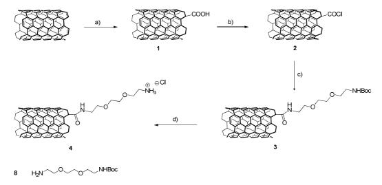
**Scheme 3.3** Synthesis of amino-functionalized MWCNTs **4**. a) H<sub>2</sub>SO<sub>4</sub>/HNO<sub>3</sub> (3:1), sonication, 24 h; b) (COCl)<sub>2</sub>, reflux, 24 h; c) **8**, THF, reflux, 48 h; d) HCl in 1,4-dioxane, overnight.
