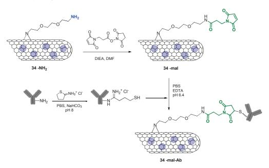
Scheme 5.10 Derivatization of amino-functionalized CNTs with the maleimide linker and subsequent coupling with thiolated Cetuximab.
