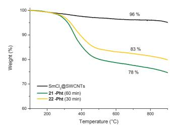
**Figure 5.6** TG curves of SmCl<sub>3</sub>@SWCNT-**B2**, phthalimide-functionalized CNTs **21** and **22** obtained by MW-assisted nitrene reaction with 60 and 30 min reaction time. Weight loss values taken at 650 °C.
