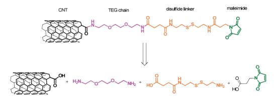
Scheme 3.1 Retrosynthetic analysis for the preparation of the CNT conjugate with a cleavable linker.
