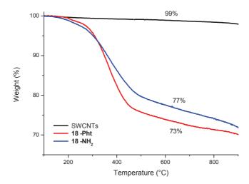
Figure 5.5 TG curves of pristine SWCNTs, phthalimide-functionalized SWCNT (18-Pht) and amine-functionalized SWCNTs (18-NH<sub>2</sub>).
