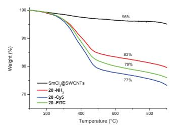
Figure 5.15 TG curves of pristine SmCl<sub>3</sub>@SWCNTs and conjugates 20-NH<sub>2</sub>, 20-Cy5 and 20-FITC.
