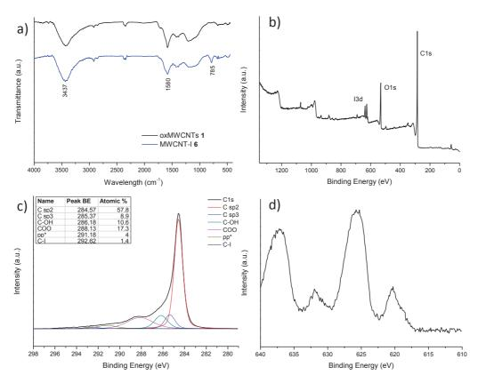
Figure 2.9 Characterization of compound 6. FT-IR (a) and XPS spectra: general survey (b), C1s (c), I3d (d).
