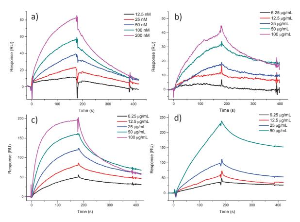
Figure 3.10 Sensorgrams showing the specific binding of: a) therapeutic nanobody (VHH), b) CNT-SS-mal-VHH, c) CNT-SS-VHH and d) CNT-VHH to the antigen  $\beta$ -catenin at different concentrations. Sensorgrams a) and d) were performed with catenin immobilized via amidation on the chip, while b) and c) were registered with biotinylated-catenin immobilized via streptavidin.
