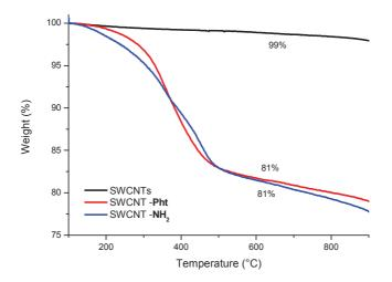
Figure 5.2 TG curves of pristine SWCNTs, phthalimide-functionalized SWCNTs and amino-functionalized SWCNTs.
