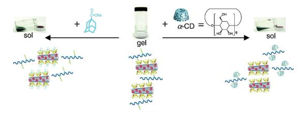
Figure 1.5 Hydrogel of SWCNTs and β-CDs prepared by  $\pi$ - $\pi$  interaction between pyrene (red) modified β-CDs (yellow) and SWCNTs (center). Gel to sol transition upon addition of a competitive guest such as adamantane carboxylate (left) and  $\alpha$ -CDs (right). Figure adapted from ref. [78].
