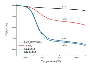
Figure 5.16 Example of TGA graph showing the curves of pristine LuCl<sub>3</sub>@SWCNTs, conjugates 33-NH<sub>2</sub>, and conjugates 33-Ab-Cy5 and 33/Ab-Cy5 obtained after 24 h incubation and dialyzed against PBS.
