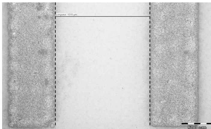
Figure 4.2: Image of Pt/YSZ/Pt sensor with measured inter-electrode distance
