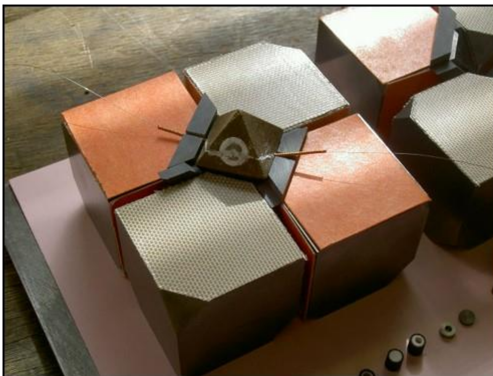
Figure III-6. Assembly for multi-anvil experiments.
