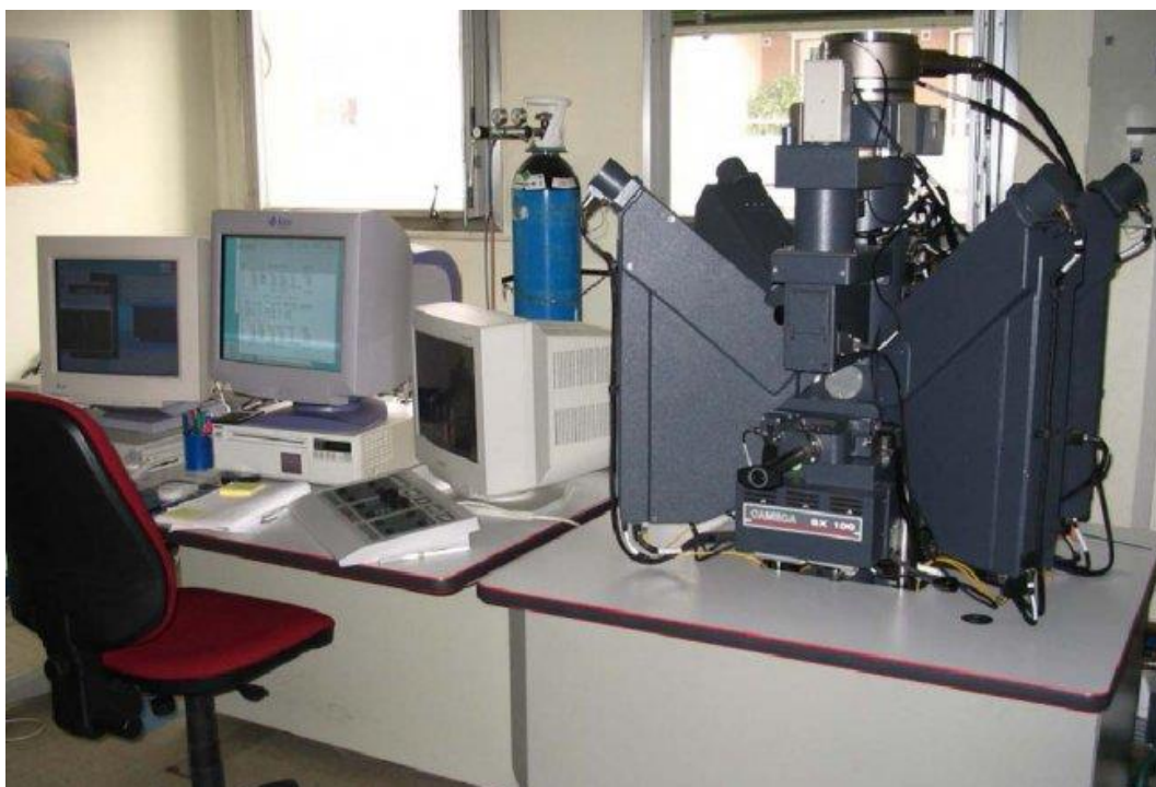
Figure III-18 : Electron probe micro-analysis at the Laboratoire Magmas et Volcans. Picture of the Cameca SX100 used to obtain chemical composition of all the mineral phases from samples produced during this thesis.
