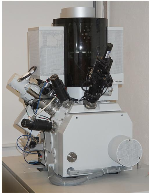
Fig. 2. 12. Helios 600 Nanolab dual beam FIB.
