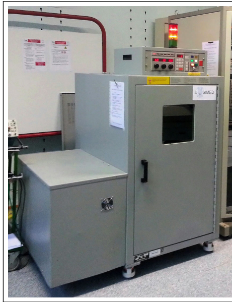
Figure 3.11 – The CP-160 Cabinet X-radiator System
