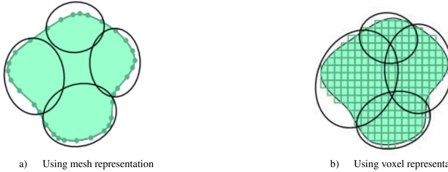
Figure 5-2 Check tumor coverage a) vertices extracted from the tumor mesh are used for the test while in b) tumor is voxelized and the inclusion of each voxel is verified [16]
