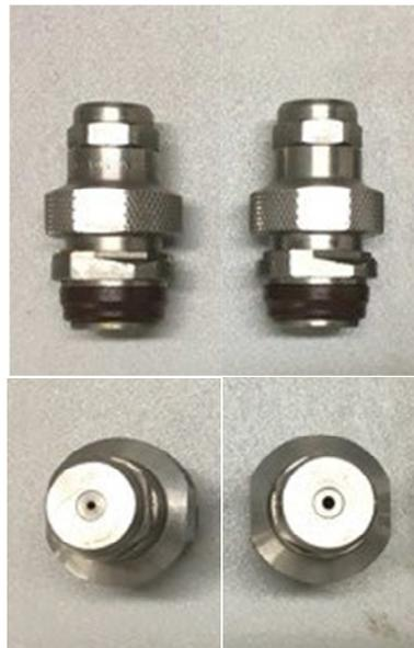
Figure 2.4 Full-cone spray nozzles (left) 0.89 mm (right) 1.50 mm
