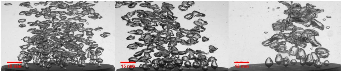
Figure 3.10 Bubbles produced at different orifice sizes at gas flow rate of 7.2 LPM
