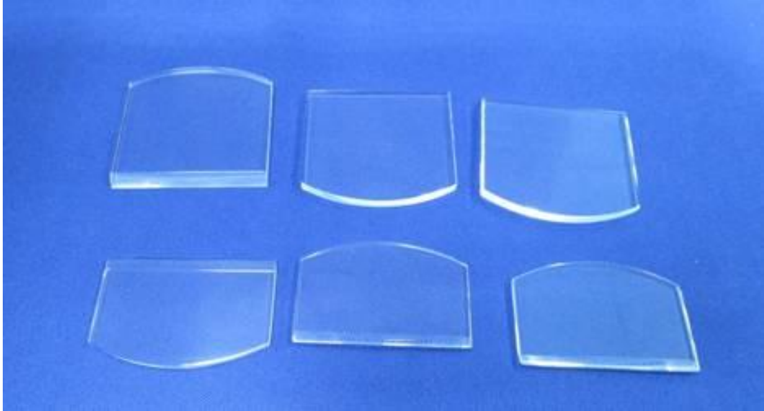
Fig. 5.1. The two waveguides have been manufactured in three pairs.
