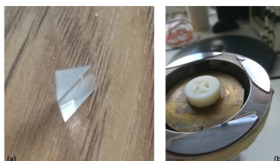
Fig. 5.11. (a) A 5 mm prism with top and bottom surfaces unpolished and (b) hand polish setup and the polished surface.
