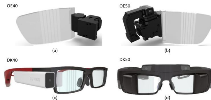
Fig. 2.35. Optical engine and development kits of Lumus [Lumus].
