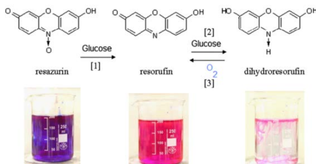
Figure 1-10. Reduction of resazurin to resorufin by glucose and sodium hydroxide (step[1]). Reduction of resorufin to dihydroresorufin by carbohydrate (step[2]). Reoxidation of dihydroresorufin to resorufin in the presence of oxygen (step[3]).
