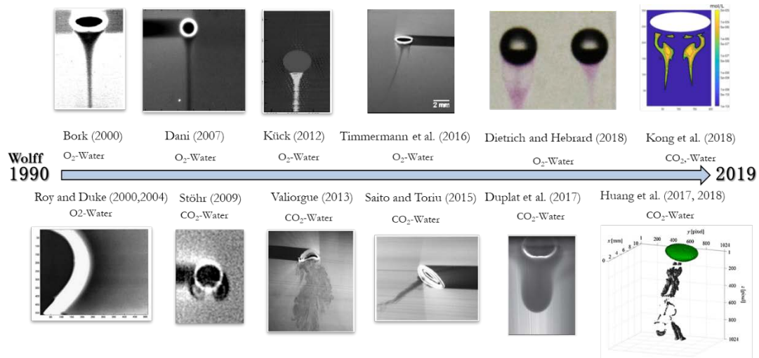
Figure 3-1 Development of mass transfer visualization of freely rising bubbles. Images from the indicated authors.
