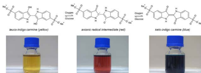
Figure 1-11. Reversible redox reaction of leuco-indigo carmine to keto-indigo carmine with glucose as reducing and oxygen as an oxidizing agent. Colour change (yellow-red-blue) is illustrated in flask experiments. Reproduced from (Krieger et al., 2017)
