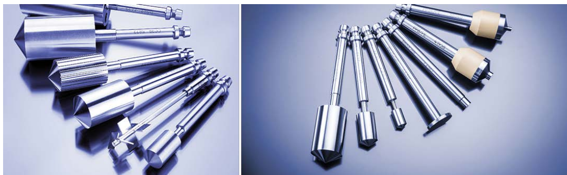
Figure 1-14 Different geometries for rheometer. Images from Anton-paar.com
