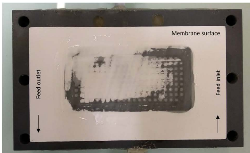
Figure C4.5 Membrane surface after wetting induced by surfactant
