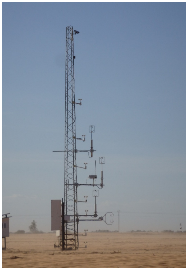
FIGURE 3.7: The main measurement (lattice) mast with the meteorological and Eddy-Covariance (EC) dust flux measurement systems. Source: Internal communication with Dr. Jean-Louis Rajot.
