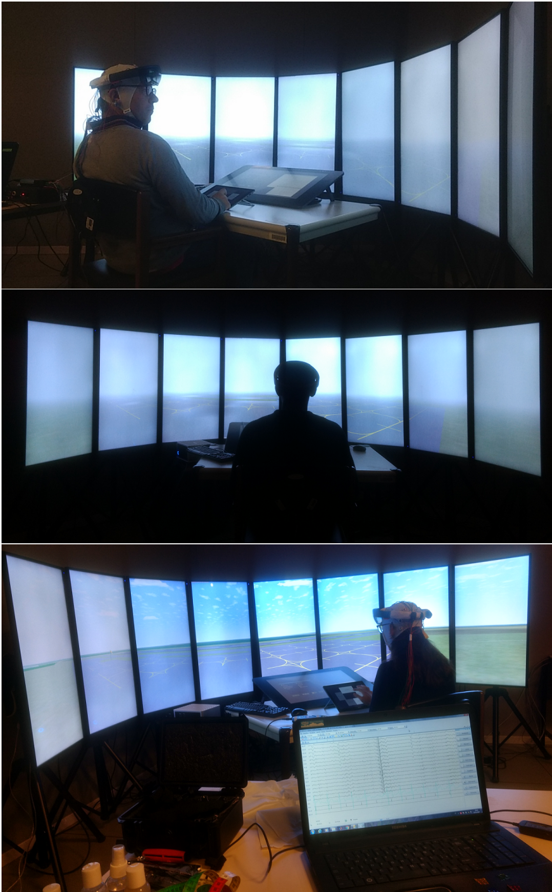
Figure 6.6 — Photograph of the sandbox used for the first experiment while a participants are answering. We can see that each participant wears an EEG on their head in the form of a cap with electrodes.
