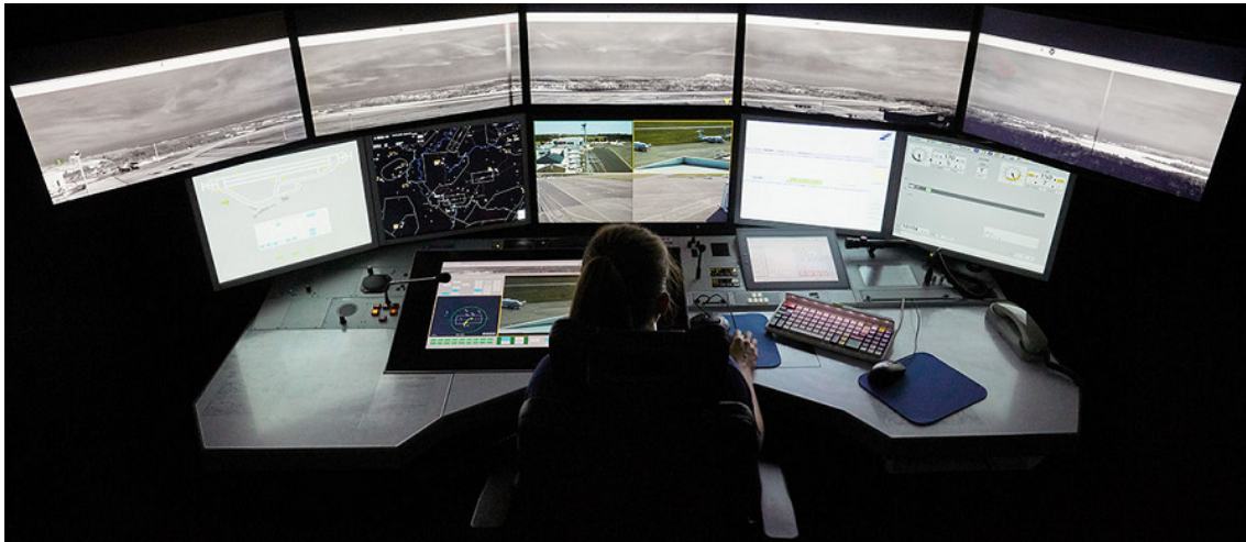
Figure 1.7 — The RCT solution used by German ANSP DFS to remotely controlled Saarbrücken airport from Leipzig.
