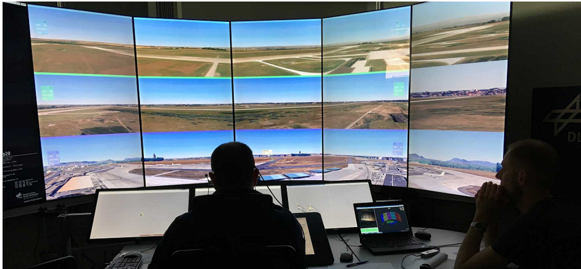
Figure 1.3 — An example of Multiple Remote Tower validation test held under SESAR 2020's PJ05 project Remote Tower for Multiple Airports in April 2018. With this exercise, 3 airports are simultaneously experimentally controlled by one ATCo.
