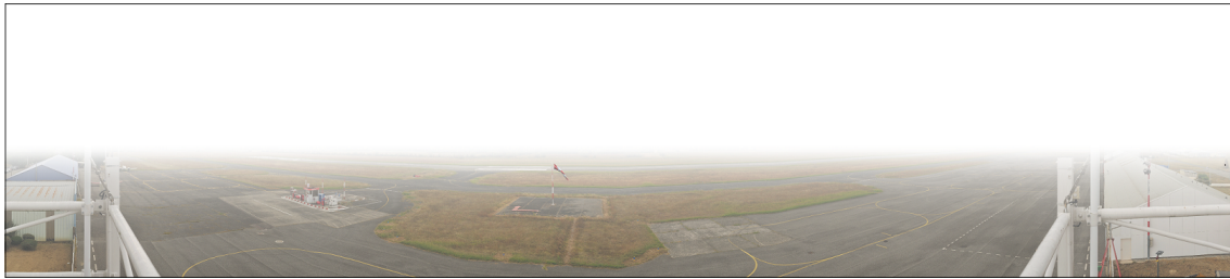
Figure 9.3 — A screen capture of the visual conditions displayed during the experiment. The fog was configured to completely cover the Muret airport runway and its environment. No aircraft were visible when they were not on the parking areas.
