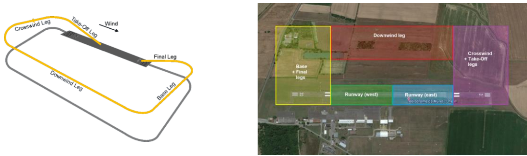
Figure 2. Generic scheme of an airport circuit (left), and discrimination of the Muret airport vicinity (right) into five distinct areas regarding this circuit.
