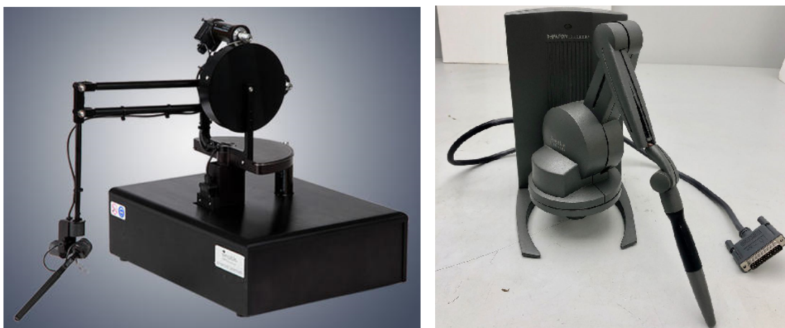
Figure 4.6 — An early model of PHANToM device (left), and a more recent one (right) [110].
