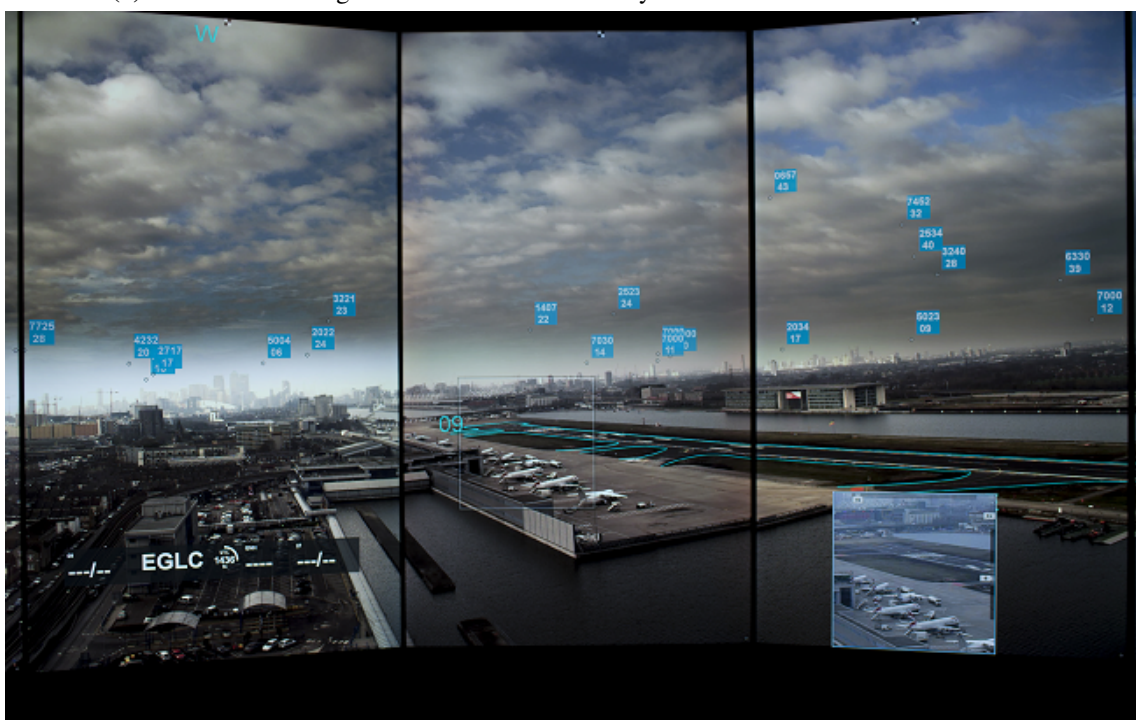
(b) Tag and zoom visual augmentation features offered by NATS RCT solution.
