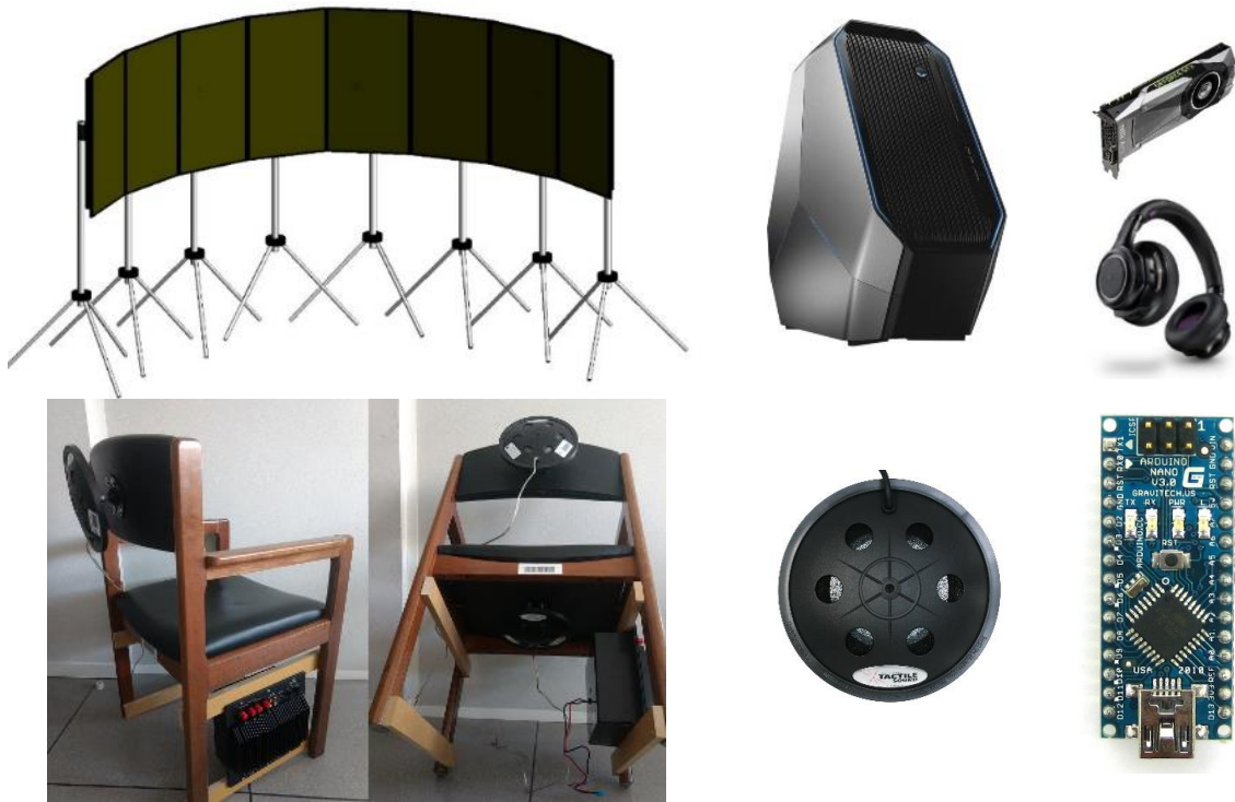
Figure 4. The 8 screens setup (top left) and Alienware Area51 computer used for the simulation (top middle) coupled with Nvidia GeForce GTX 1080 graphic card (top right top) will display FG graphical environment. Plantronics BackBeat Pro stereo headphones (top right bottom) will play spatialized engine sounds, and the haptic chair set up (bottom left) will give up and down cues through vibrotactile feedbacks using two ClarkSynthesis T239 Gold transducers (bottom middle). An Arduino Nano microcomputer associated to an IMU (bottom right) will retrieve the participant head orientation.
