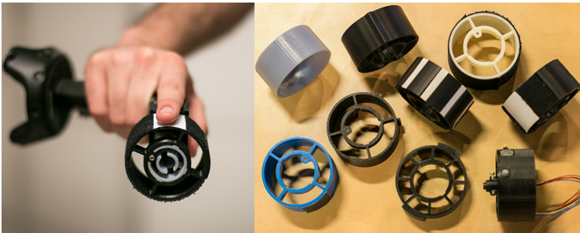
(b) The Haptic Revolver providing texture sensation on geometrical objects explored by the user.
