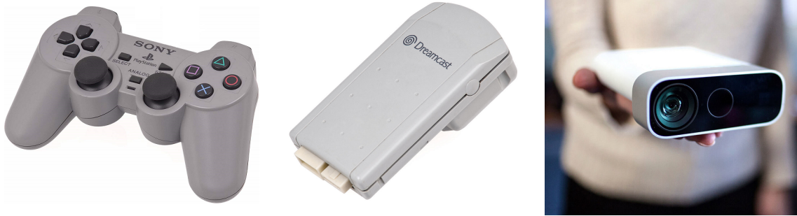
(a) The Sony DualShock 1 game controller used in early versions of PlayStation 1 console (1997). (b) The Sega vibratory kit which could be plugged into the Dreamcast game controller (2000). (c) The new Microsoft Kinect device, used to capture body's movements (2019).
