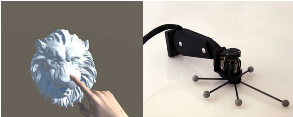
(a) The NormalTouch haptic device providing cutaneous sensation on the fingers by means of force feedback and vibrations.
