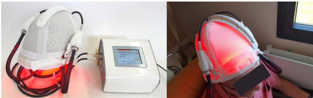
Figure 1. The fabric-based biophotonic device used for P-PDT: red light is emitted by an optical fibre-based fabric that lines the inside of a cap, which is held in place by an ergonomic helmet.
