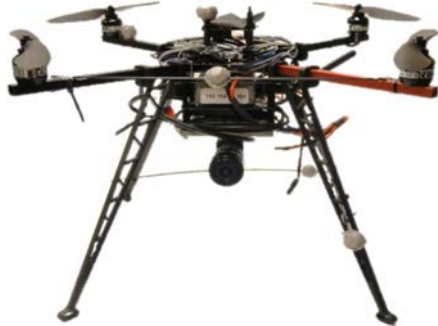
(a) Drone MK-Quadro de MikroKopter.
