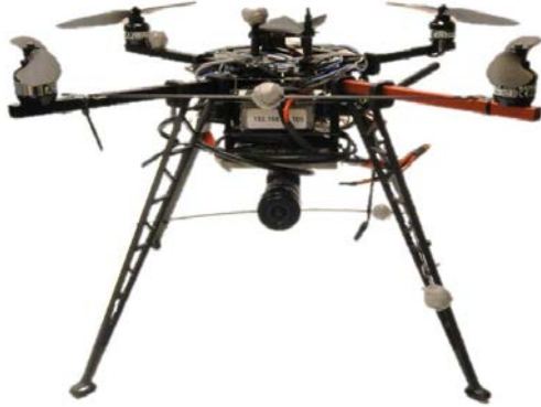
(a) Drone MK-Quadro de MikroKopter.
