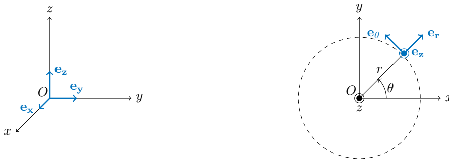
Figure A.1: Left: Cartesian coordinates (x, y, z) . Right: Cylindrical (polar) coordinates (r, \theta, z) .
