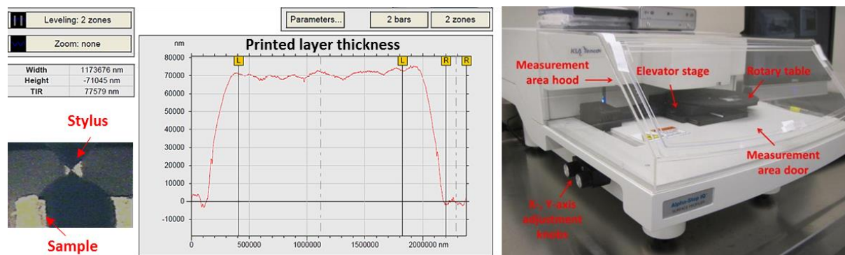
Figure III-2: Example of thickness profile (left), and Tencor contact profilometer used at IMS (right) laboratory.
