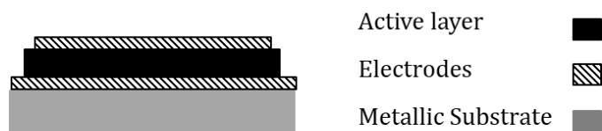
Figure IV-7: Scheme of the multilayer considered as the “elementary brick” of the EH structure.
